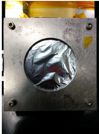
Figure 3.9: Image of the fast plastic scintillator (BC-408) mounted in its custom housing with mylar windows installed. The Hamamatsu R1635 photomultiplier tube is typically mounted to the windows on the left or right hand side of the housing (not shown).
