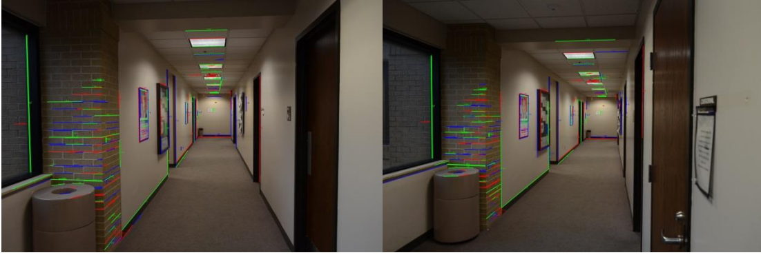
Fig. 5 175 line segments are matched for two image views for same scene
