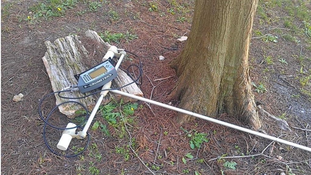
Figure 12 - Typical set up of the G-858 Magnetometer in vertical gradiometer mode
