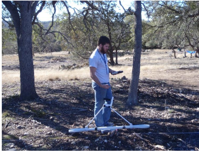
Figure 15 - Charles Stanford demonstrating typical setup of the EMP-400 system
