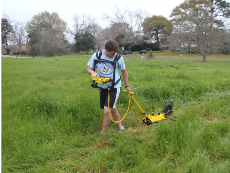
Figure 16 – Charles Stanford demonstrating typical setup of the PulseEkko system
