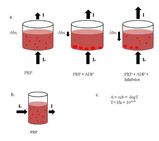
**Figure 4**. The Mechanics Behind Absorbance Readings. This diagram explains the problem with the data gathering of the plate reader. Light passes vertically in the plate reader (a.), so when clots sink to the bottom they affect the readings. PRP+ADP would have had a much lower absorbance if the reading was taken horizontally like in an aggregometer (b.) The equations to the side of this figure (c.) also help explain the logic behind absorbance and transmittance.
