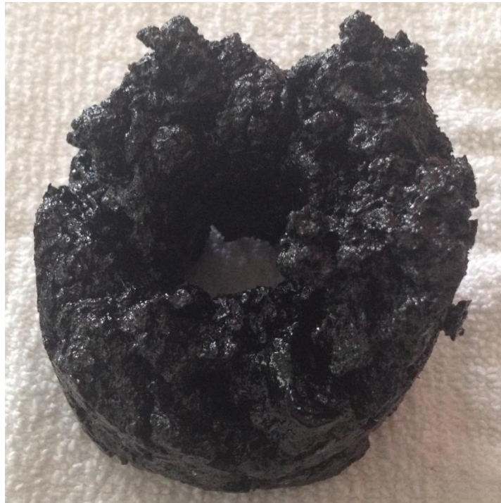
Figure 12. First novel aluminized prototype hybrid motor curing test.
