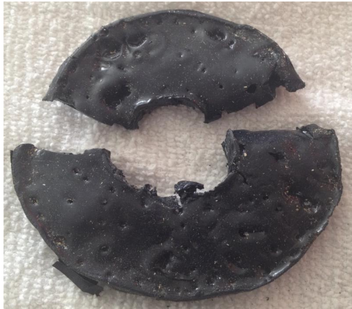
Figure 13. Second novel aluminized prototype hybrid motor curing test.
