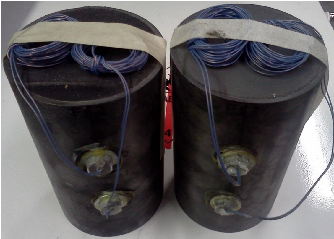
Figure 9. Representative plain HTPB (left) and aluminized (right) experimental motors with a length and diameter of 6 and 3.375 inches, respectively, and a combustion port diameter of 1 inch. MIRRAS sensors are embedded 2 inches from either end and are mounted perpendicular and tangent to the combustion port surface.
