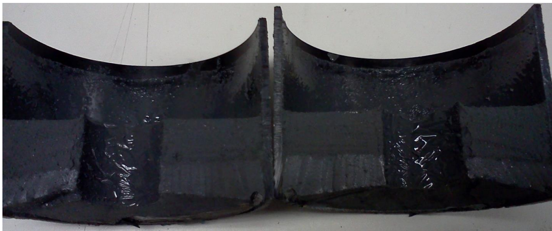
Figure 8. Commercially aluminized hybrid motor prototype after curing.
