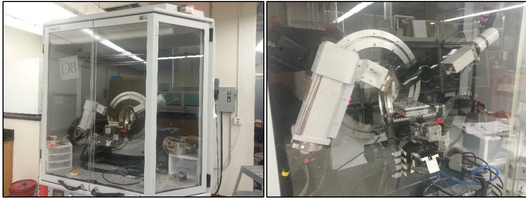
Figure 3-5. Bruker D8 Discover instrument used for XRD analysis.
