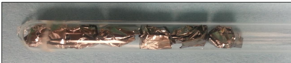
Figure 3-3. Sealed quartz tube before homogenization or annealing. Tube contains 3 samples each of 6 alloys (L to R: U-7Mo-2Zr, U-7Mo-5Zr, U-7Mo-10Zr, U-10Mo-2Zr, U-10Mo-5Zr, U-10Mo-10Zr).
