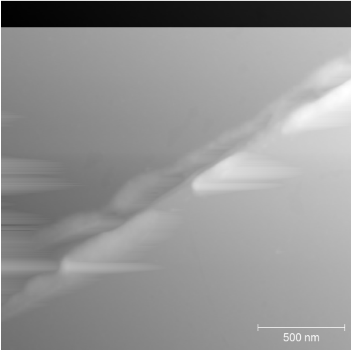
Figure 4.7: AFM image of the sample surface from Figure 4.6, the surface was seen to be flaking (the diagonal blurry lines) and would be rejected from further processing.
