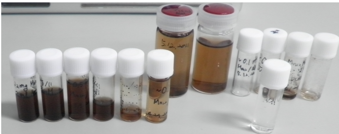
Figure 3.4: This is a series of sample solutions made while doing iterative testing for sample improvement. In particular I was attempting to find an upper bound of solubility of Mn_{12} -Ph in benzene.
