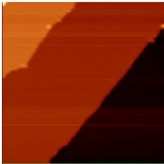
Figure 2.8: \approx 150 nm x 150 nm, showing four distinct terrace steps of Cu(111) allowing for precise \hat{z} -piezo calibration. The tunneling current was 150 pA and the sample bias was -300 mV. This work was done in collaboration with Patrick Han.
