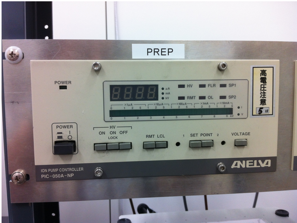
Figure A.2: This is the Ion Pump Controller panel, located above the STM controller.
