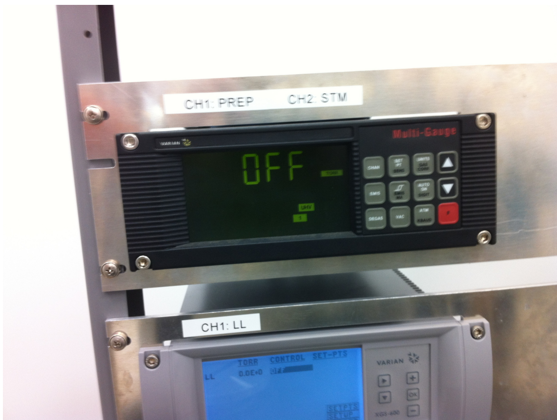
Figure A.3: This is the pressure gauge for the sample-prep chamber, located above the gauge for the load-lock chamber.
