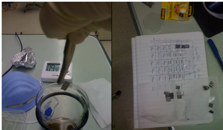
Figure 3.1: Dipping and drying samples for shipment and testing in a UHV STM in Japan. These samples were on exfoliated pyrolytic graphite (which is very hard compared to HOPG) and had droplets of Mn_{12} -Ac in Acetonitrile ( CH_3CN ) added to the surface.
