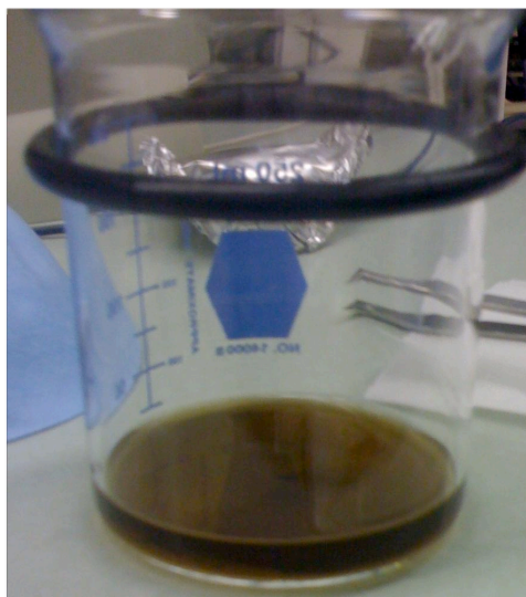
Figure 3.2: An example solution using the older methodology. You can see a uniform, dark, liquid. These solutions required high density to assure that the density on molecules on the graphite surface would be high enough to find via STM within a reasonable time. Operating near the saturation point of the solvent meant that care had to be taken to not drop any sedimentation which was present in the solution onto the sample surfaces.
