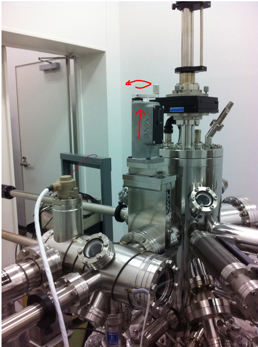
Figure A.1: This is the gate valve between the load-lock and sample-prep chambers.
