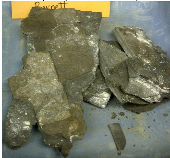
Figure 2.6 – The Barnett outcrop sample used for the experiments in this study.
