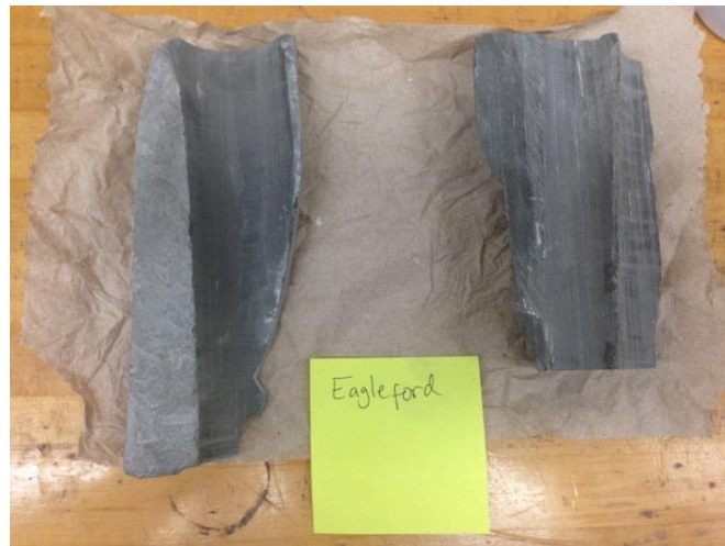
Figure 2.8 – Eagle Ford shale outcrop used for this project.
