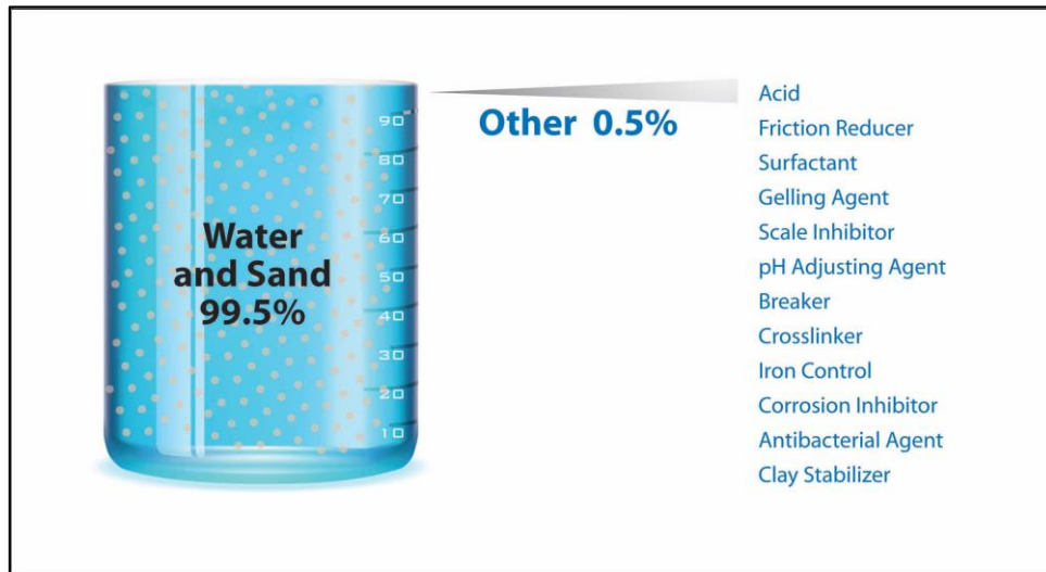
Figure 2.12 – Composition of a typical gel fracture fluid.
