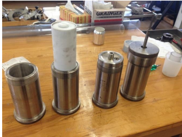
Figure 3.8 – The Aging Cells used in the experiments.
