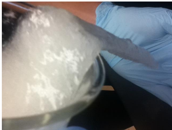
Figure 3.6 – Fully cross-linked gel fracture fluid. Lipping characteristic is observed.
