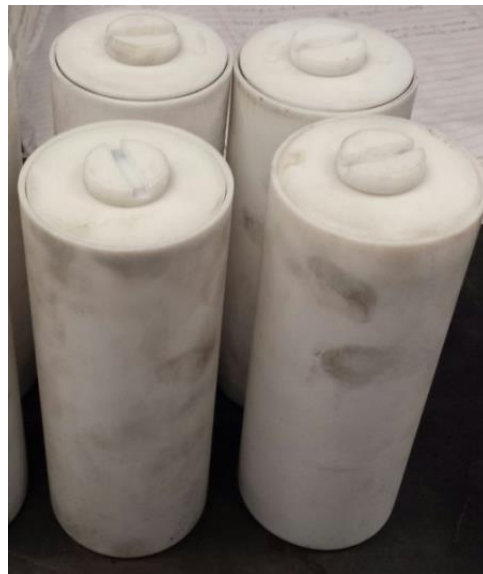
Figure 3.9 – Teflon liners that go in the Aging Cells.
