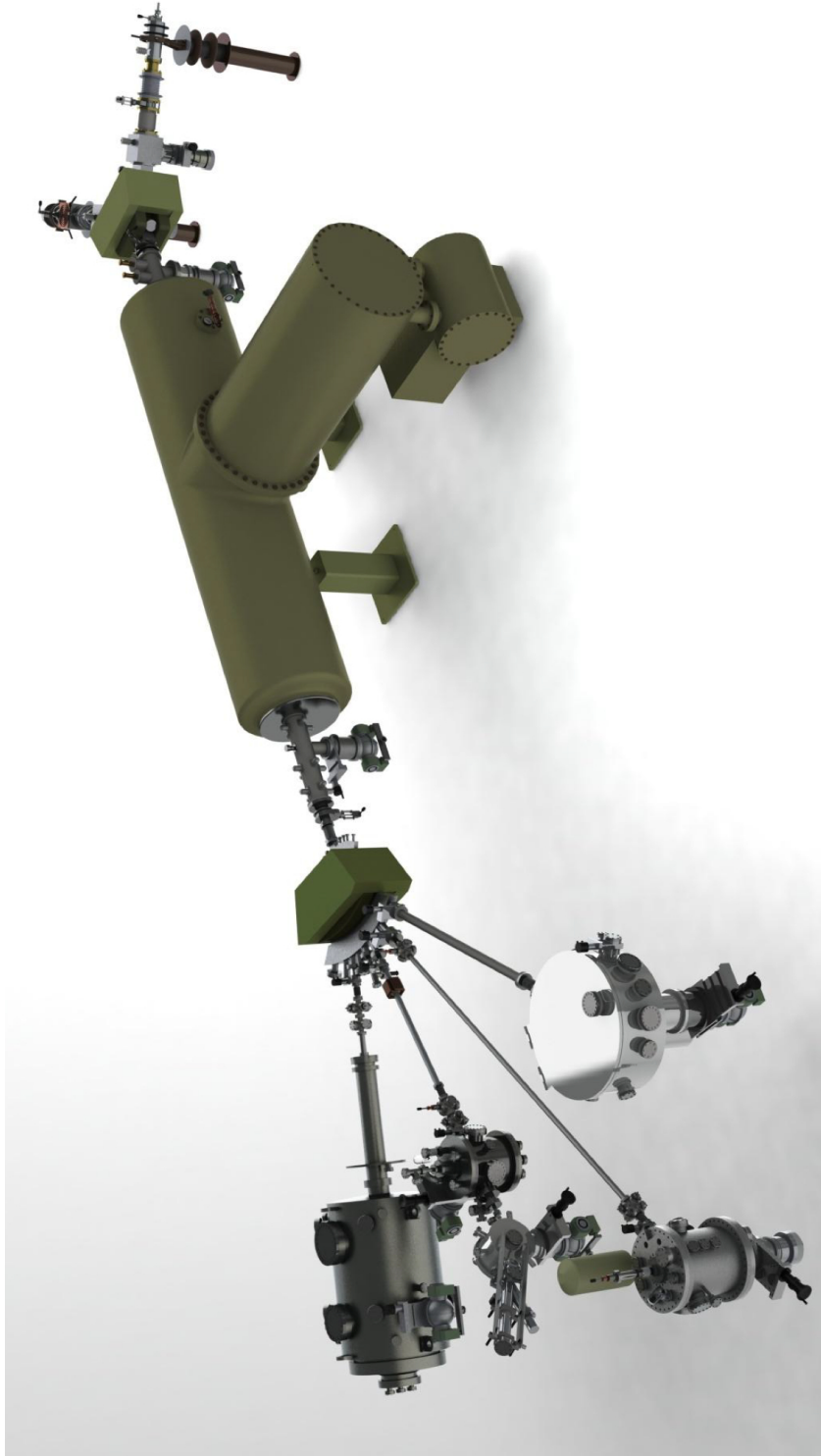
Figure 2.6: A schematic of the 1.7 MV tandem accelerator at Texas A&M University. From right to left are the two ion sources, followed by a low-energy mass-selection magnets, T-shape tank with high voltage terminal, a quadrupole lens and a high-energy magnetic mass analyzer. Two major beam lines shown here: the implantation chamber with temperature control shown as second beam line and the analysis chamber shown as the third beam line.
