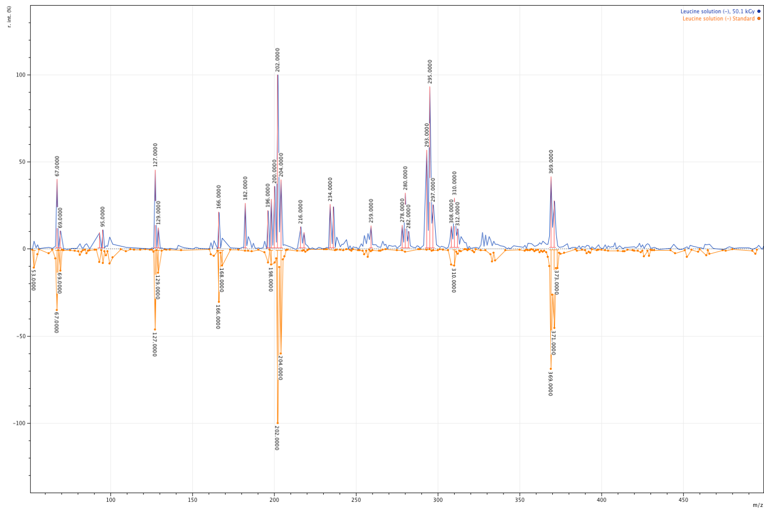
Figure A.62. ESI-MS spectrum of leucine in aqueous solution for control and irradiated 50kGy samples: negative mode
