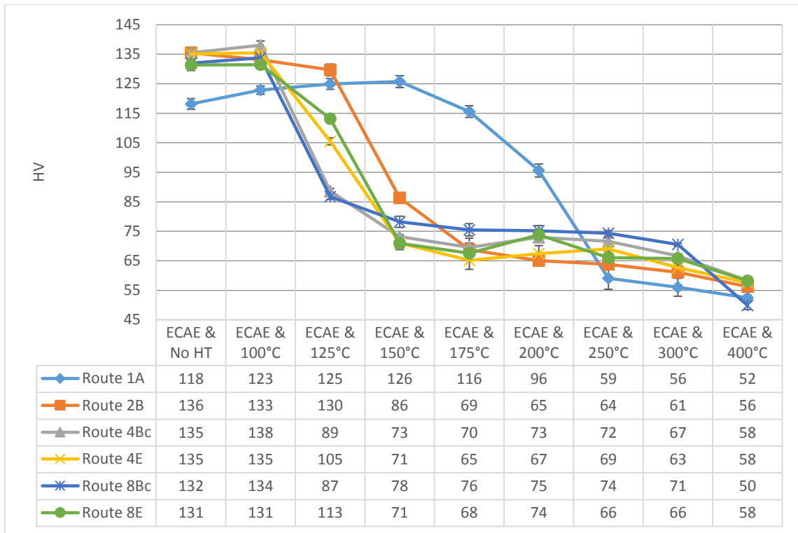
Figure 14. The hardness of copper C101 after ECAE and one-hour heat treatment at different temperatures.
