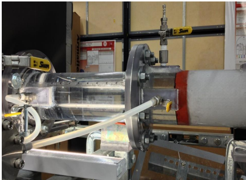
Figure III.3. 4. Filter Bag in the high temperature horizontal test facility
