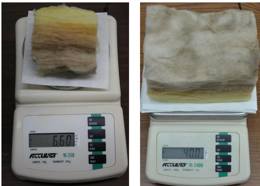
Figure III. 1. 4. Debris final quantity – 6.6g (left), 40g (right)
