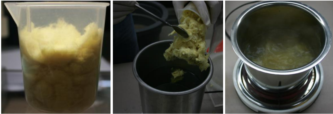
Figure III.1. 1. Debris preparation using shredder method (a) NUKON prepared using a leaf shredder and (b) and (c) boiled for 10 minutes in 2-liter stainless steel jar
