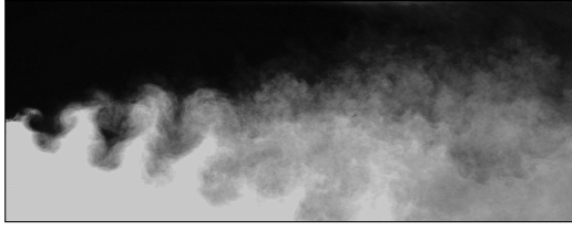
(a) \rho^* for case 8: (\lambda_1, \lambda_2, \beta) = (8 \text{ cm}, 2 \text{ cm}, 45^\circ) , (b) \chi^* for case 8: (\lambda_1, \lambda_2, \beta) = (8 \text{ cm}, 2 \text{ cm}, 45^\circ)
