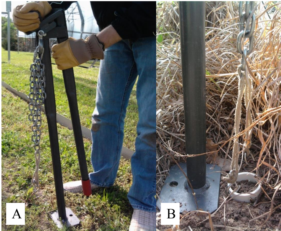
Fig. A.12 Tools used to install N mineralization incubation core; (A) T-post puller with rope, chain, and s-hooks designed to lift the apparatus (B) PVC cores from the ground without disturbing the sample or surrounding soil.
