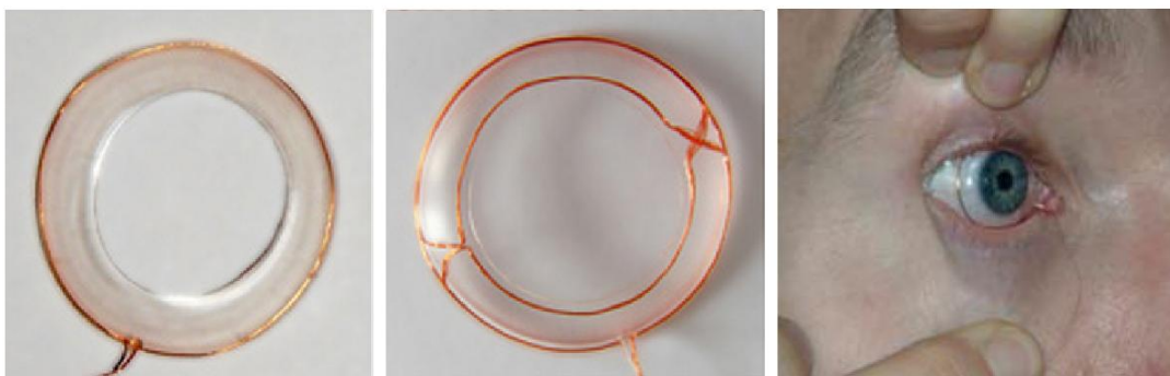
Figure 8. Scleral search coils contact lens. ( http://www.chronos-vision.de )
