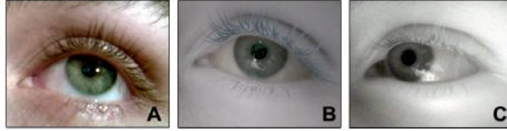
Figure 13. Image captured by a webcam. (A) With IR filter only. (B) With IR pass filter only. (C) With IR pass filter and illuminate by IR LED. (Mantiuk and others 2012)
