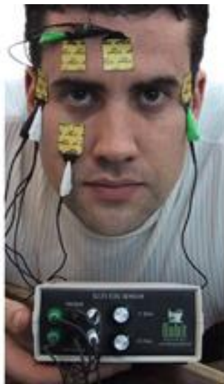
Figure 7. Electrodes of EOG placed around the eyes. ( http://www.qubitbiology.com )
