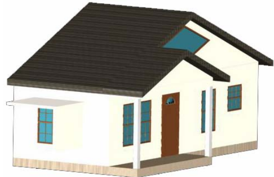
6L – Maximum 6-foot overhang with vertical fin and with clerestory window
