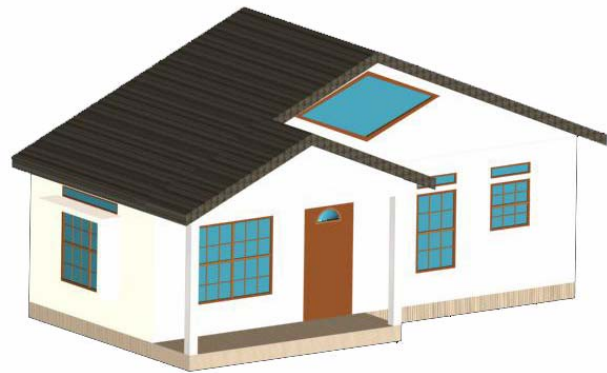
10L – High window with 18-inch overhang with vertical fin and with clerestory window
