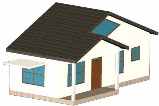
4L – Maximum 6-foot overhang with clerestory window
