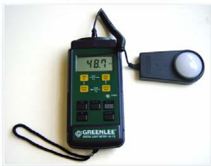
The reference light meter (model 93-172)
