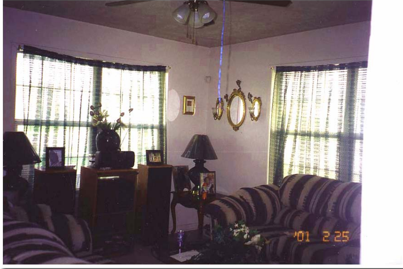
Figure 3.9 – Photograph of the living area. It can be seen from the photograph that the occupants tended to keep the curtain drawn almost all day due to privacy concerns. Therefore, the need for using electric lighting during daytime resulted in high consumption of lighting energy during building occupancy.
