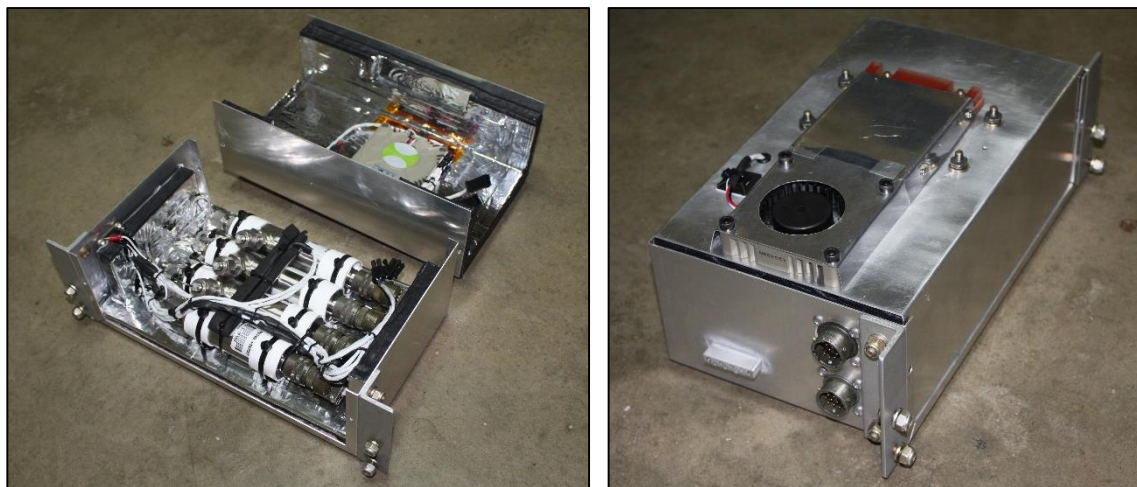
Fig. 58 Temperature-controlled pressure-transducer box, a) inside box, b) outside box
