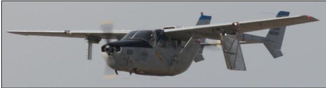
Fig. 17 Cessna O-2A with SWIFTER attached to the port, outboard hardpoint and the hotwire sting mount attached to the starboard, outboard hardpoint
