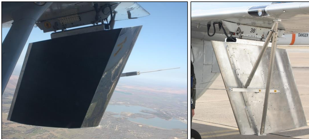
Fig. 18 SWIFTER attached to O-2A, a) test side of SWIFTER and five-hole probe (5HP) (pilot perspective), b) non-test side of SWIFTER with dual-strut assembly and 5HP
