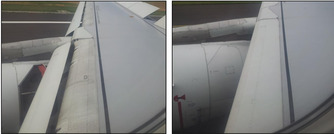
Fig. 1 Airbus 319 leading-edge slats during landing, a) slats deployed, b) slats retracted
