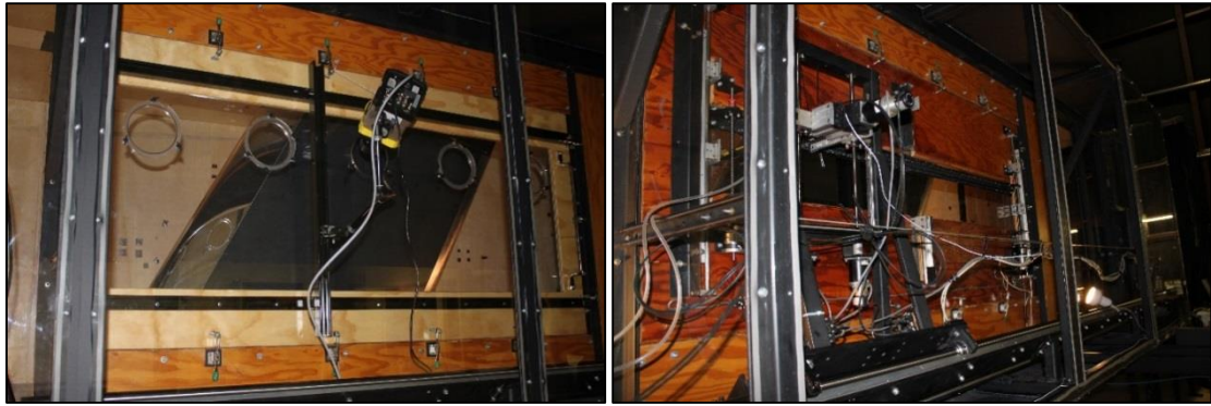
Fig. 23 SWIFTER installed in KSWT, a) infrared thermography setup, b) hotwire traverse setup
