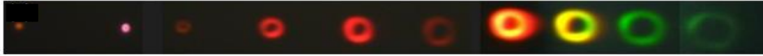
Figure 7 Adjusting the power of pump and Stokes. When the intensity of the pump and Stokes beams are attenuated, low-order sidebands OV's have symmetric beam profiles; OV are ready to be measured.
