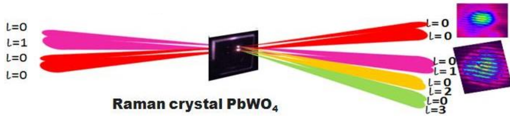
Figure 12 Two pairs of beams are focused in different part of a Raman-active crystal—PbWO 4 . The beams are close and overlap partially. The interference of the beams occurs and gives the phase profiles of the optical vortices.
