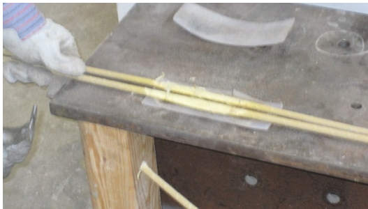
(c) Resin softened and pliable
