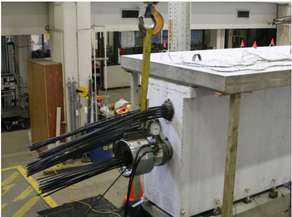
(b) Post-tensioning jack and strands
