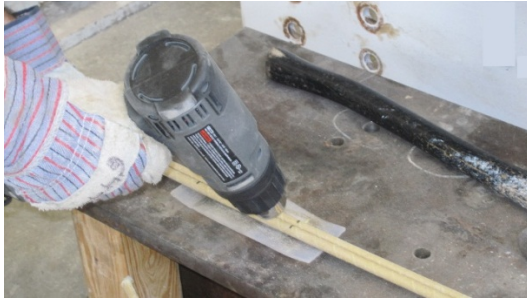
(a) Heating the resin
