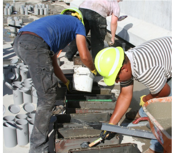
(b) Making MOR beam samples
