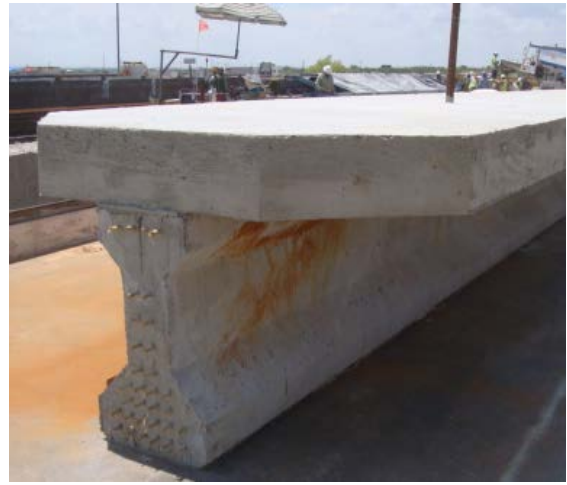
(b) Girder with composite deck
