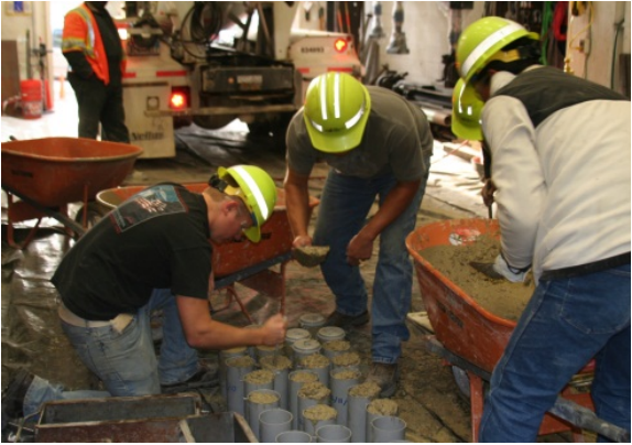
(a) Making cylinder samples
