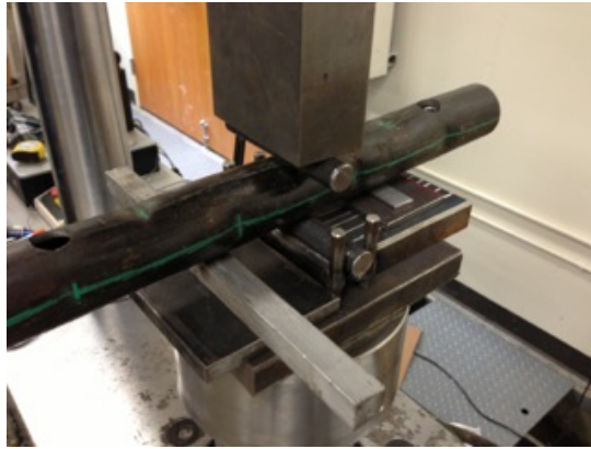
Figure 4.8. Crimping Pipe Every 2 in. at 90° Turns.
