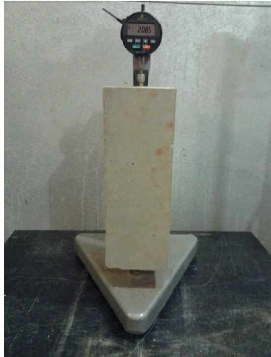
(b) Measuring shrinkage of the sample
