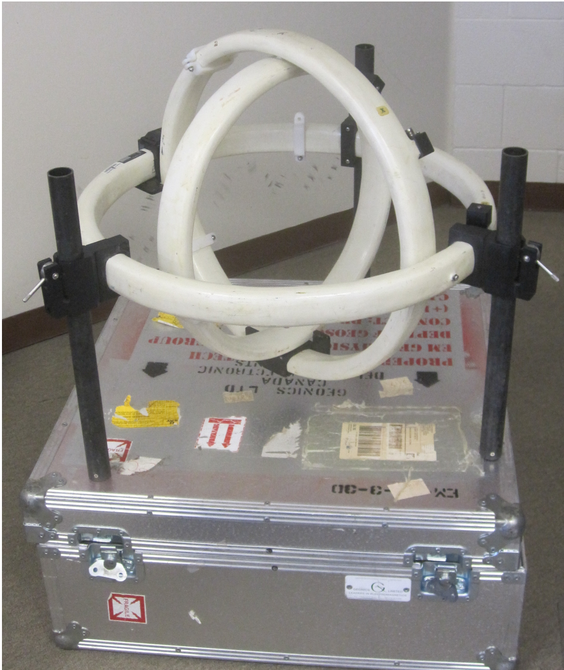
Figure 4.2: The receiver coil used in this study is shown. There are 3 separate coils in order to measure the x , y , and z components of the magnetic field produced by the subsurface currents.
