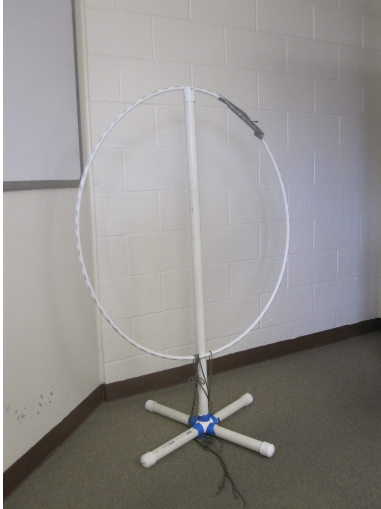
Figure 4.1: The 3-D source used for data acquisition in Mason, TX. The wire loop used to create the magnetic field is threaded through the circular PVC pipe. The loop can be rested on the top of the stand (as shown above) for either the x or y orientations, or it can be suspended from the top of the stand in a horizontal position for the z orientation.
