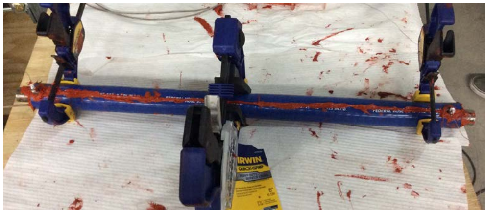
Figure 3-16: Sealing the heating tapes with silicon tubing and adhesive
