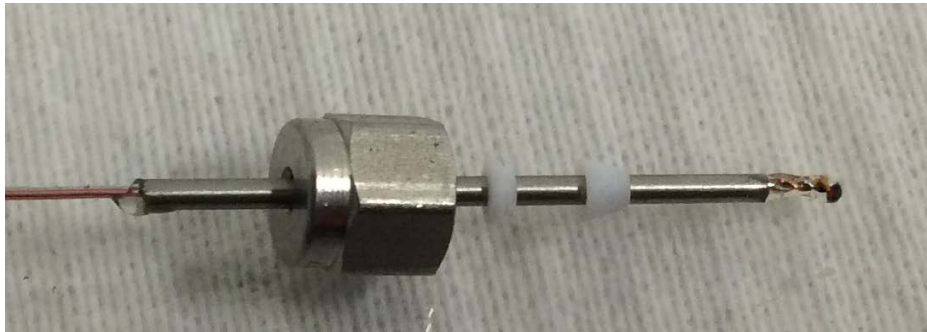
Figure 3-17: Thermocouple with tubing, epoxy, and ferrules
