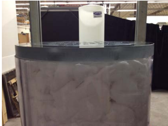
Figure 3-12: Top plate flush with containment
