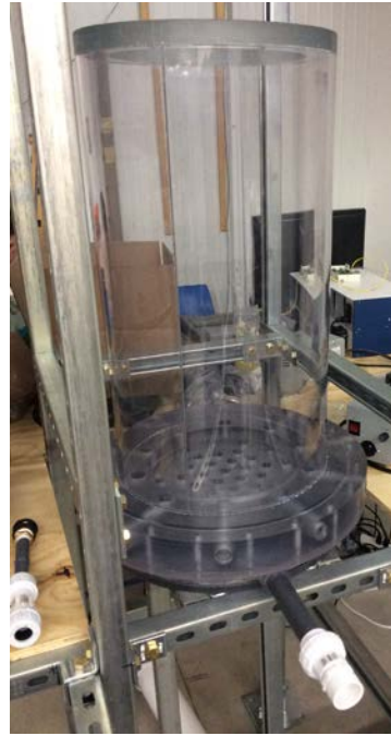
Figure 3-8: Lower plenum and core containment
