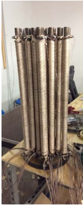
Figure 3-7: Piping, heating tape, and thermocouples
