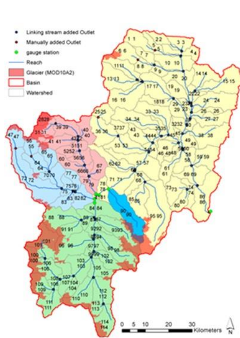
Figure 1. 13. Subbasins delineation, glaciers outlines, and locations of dams and flow gauge stations in Mendoza River Basin. The flow data from colored subbasins is used for model calibration.
