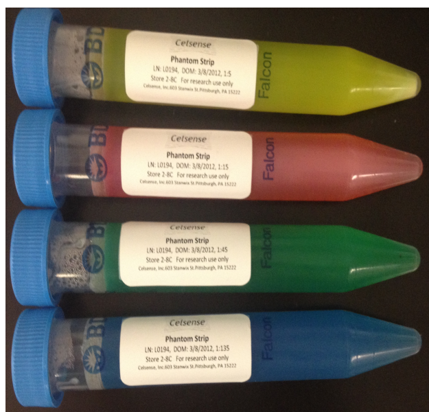
Figure 7: Cell Sense 10 mL phantoms in decreasing fluorine-19 strength from top to bottom.
