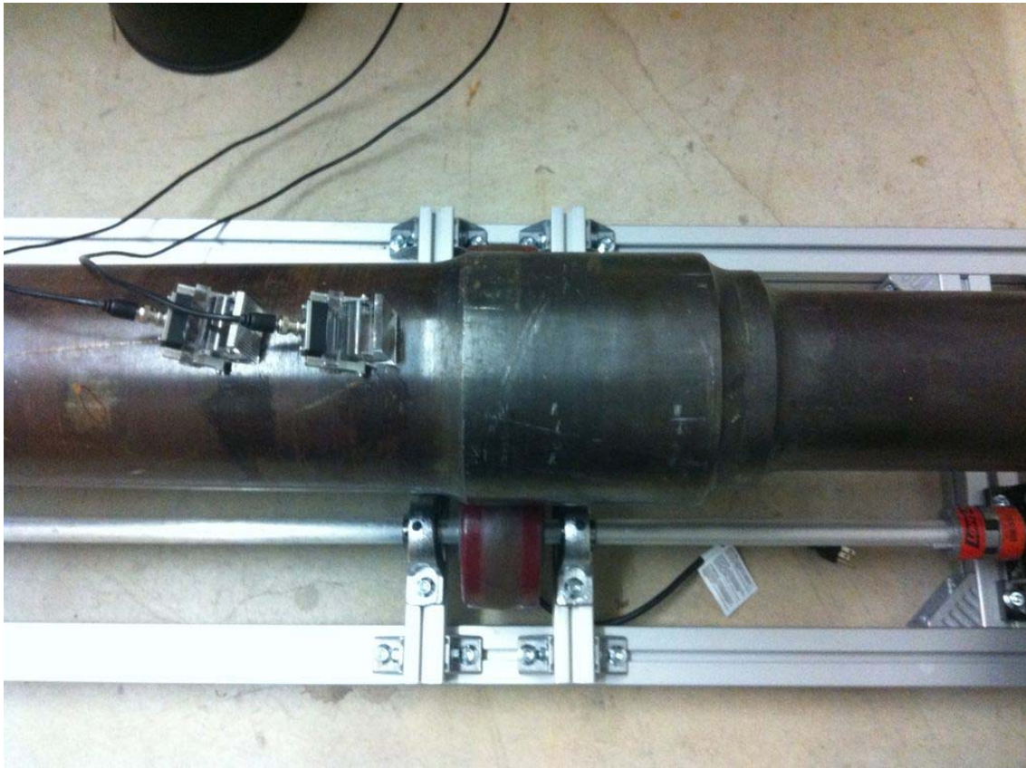
Figure 6.5. Transducers placed on one side on the same line
