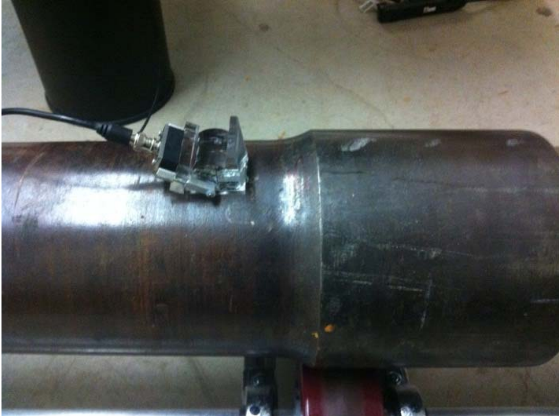
Figure 6.1. Experimental setup of pulse-echo mode [10 in. (254 mm) apart from the transducer to the defect]
