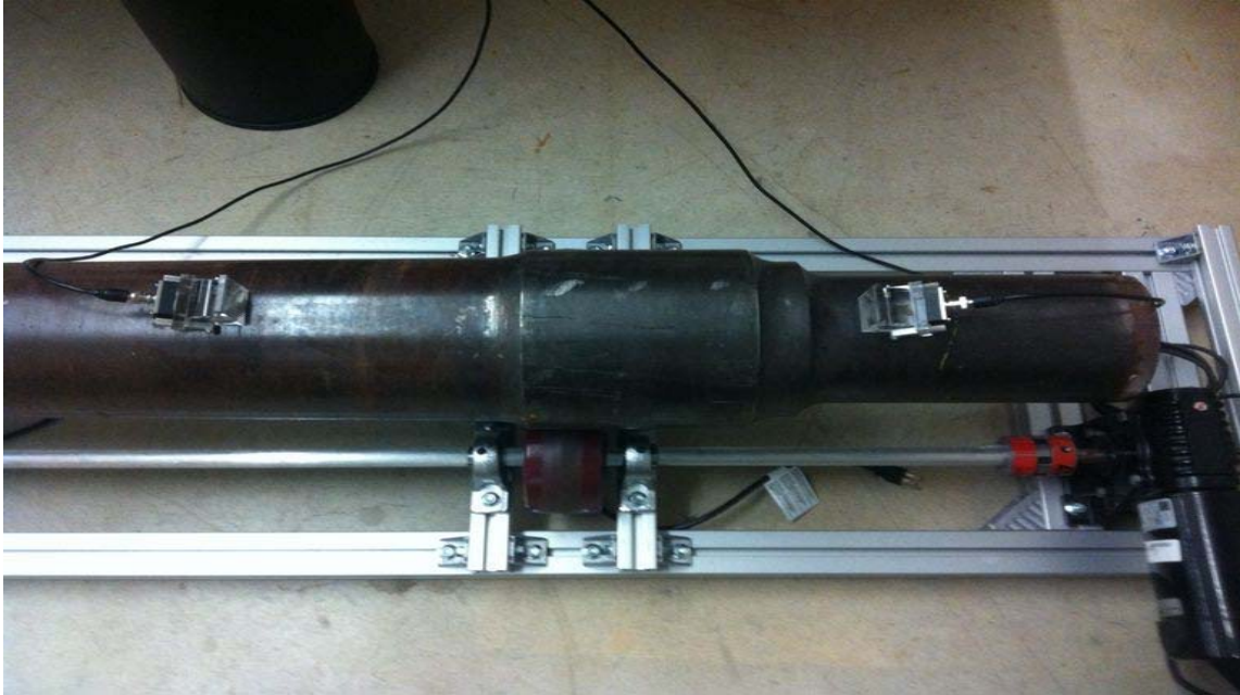
Figure 6.3. Transducers placed facing each other [20.5 in. (520.7 mm) apart from the transmitting transducer to receiving transducer]
