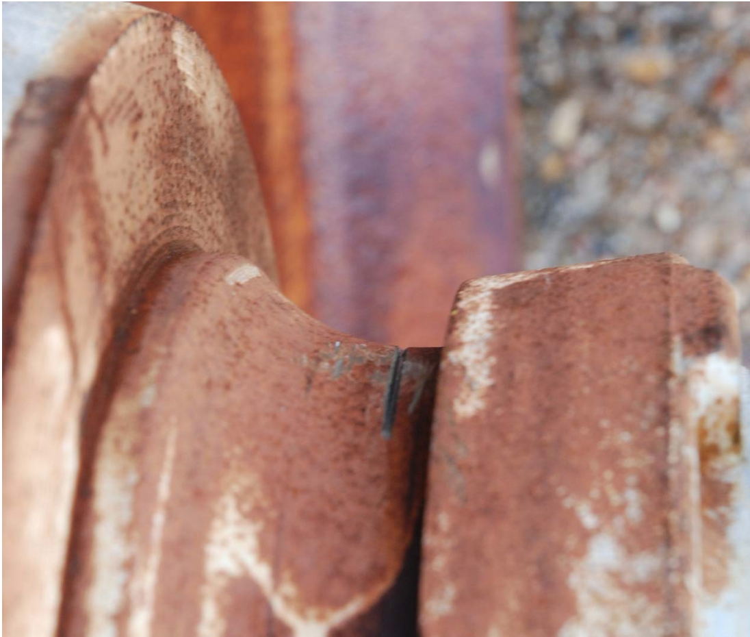
Figure 5.13. Artificial crack using cutting wheel
