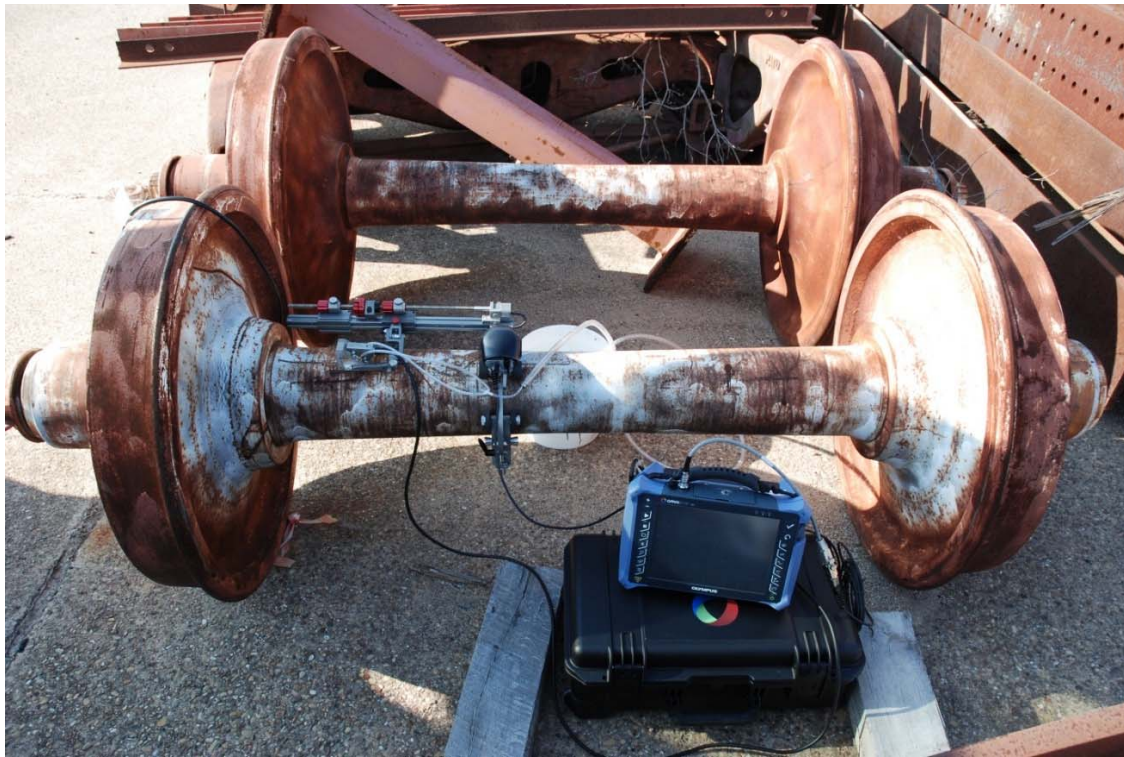
Figure 5.11. TTI axle scan setup
