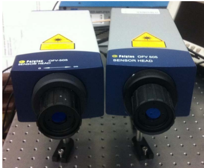
Figure 7.31. Laser array system
