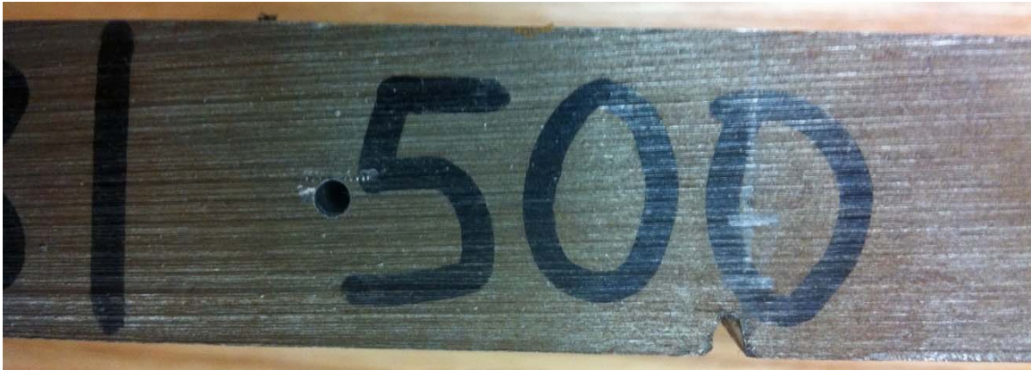
Figure 7.32. Discontinuity of the test specimen
