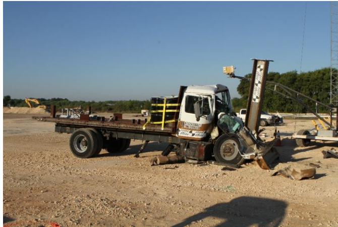
Figure 3-71: Medium duty truck and pile after the impact (M50)
