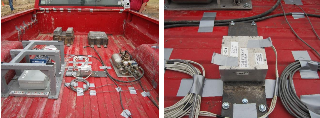
Figure 3-7: Accelerometer, angular rate transducer, and data acquisition on a pickup truck rear
