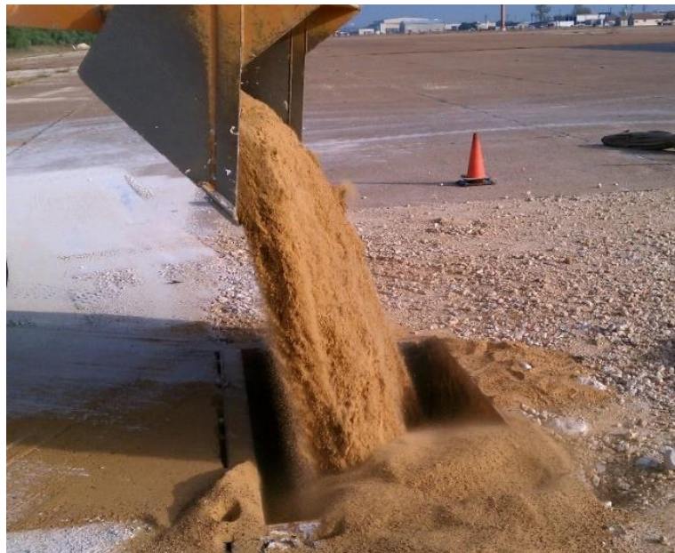
Figure 3-22: Pouring sand into the test box
