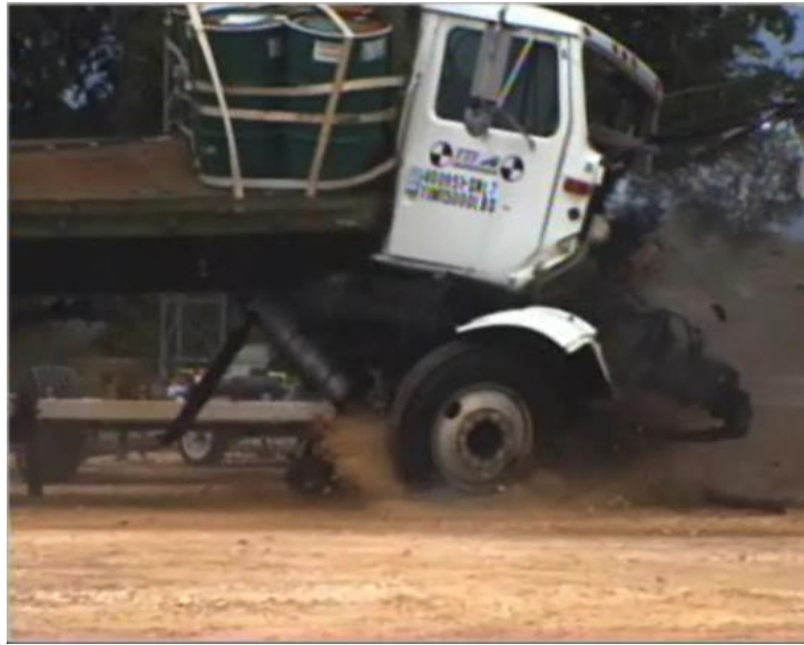
Figure 3-12: Impact frame captured from high speed camera of K-12(M50) test (Alberson et al. 2007)
