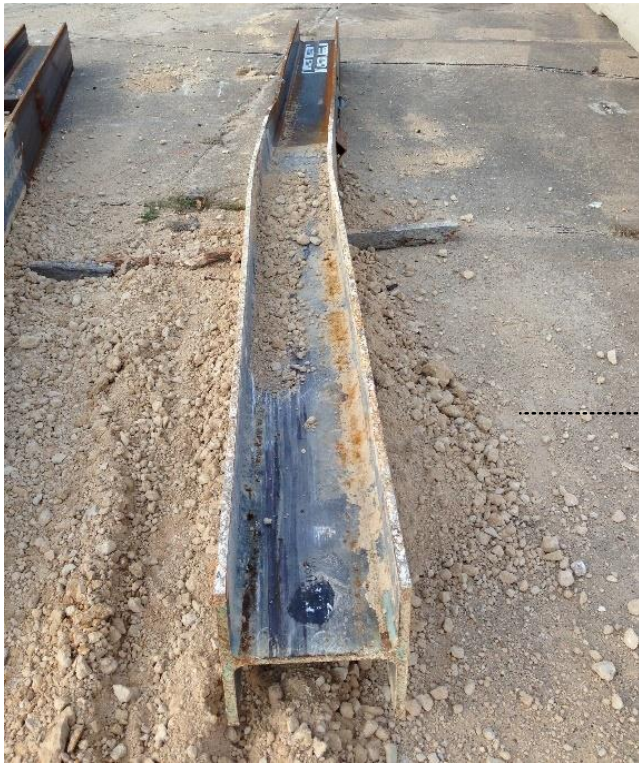
Figure 3-73: Pile plastic deformation after the M50 (unit is meter)
