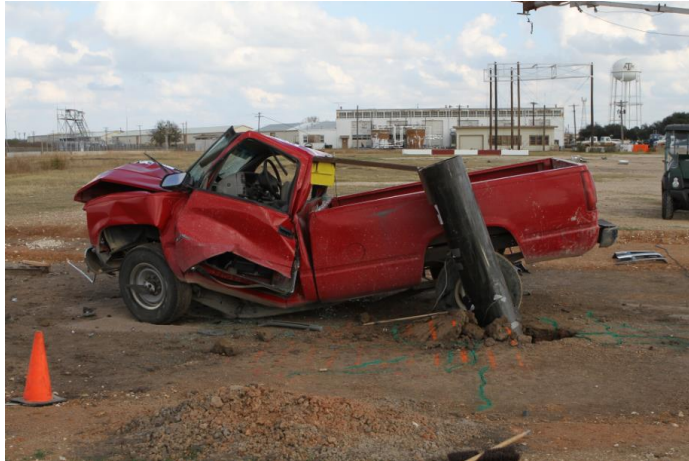
Figure 3-58: Pickup truck and pile after the impact (PU60)
