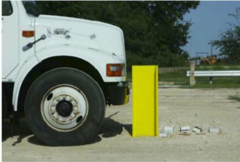
Figure 3-11: Full-scale K-12(M50) impact test on single post (Alberson et al. 2007)
