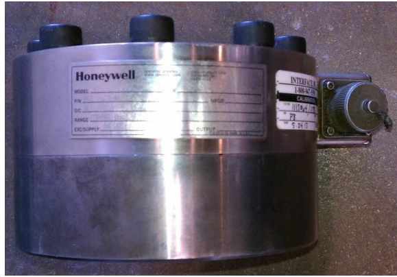
Figure 3-2: Load cell used for PU60 static test
