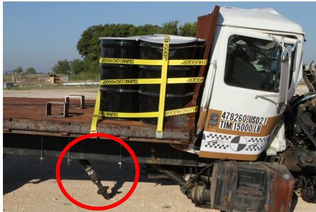
Figure 4-16: Broken shaft in the M50 test
