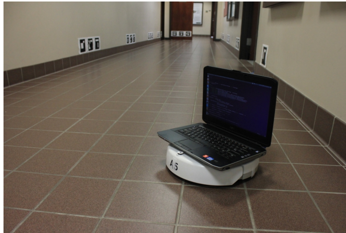
Figure 8.2: A picture of the robot (an iRobot Create) in the operating environment. Landmarks can be seen on the walls.
