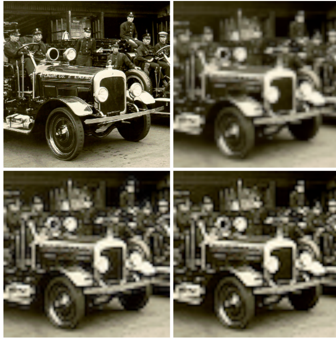
Figure 7.3: An example of a high-resolution image (top left) downsampled using a box filter (top right), optimized for bilinear reconstruction (bottom left), and optimized for bilinear reconstruction constraining values to [0,1] (bottom right).
