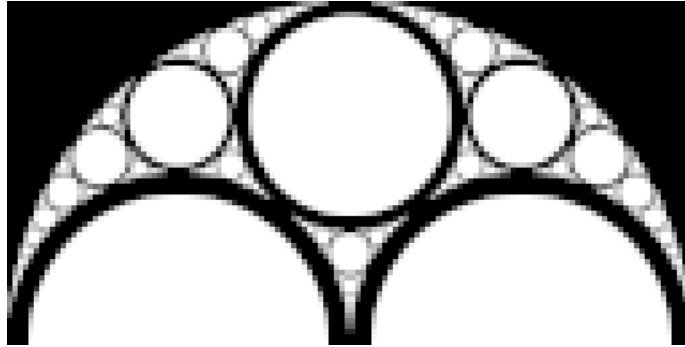
Figure 2.7: Rasterization of rational Bézier curves of varying sizes in a 128 \times 64 pixel image.
