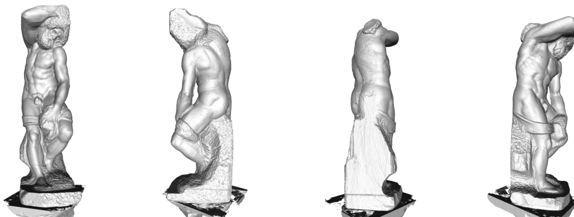
Figure 4.1: Surface reconstruction of “Barbuto” from laser range scans containing a total of 329 million points (7.34GB of data). Our wavelet surface-reconstruction method completed the reconstruction in 112 minutes with 329 MB of memory.
