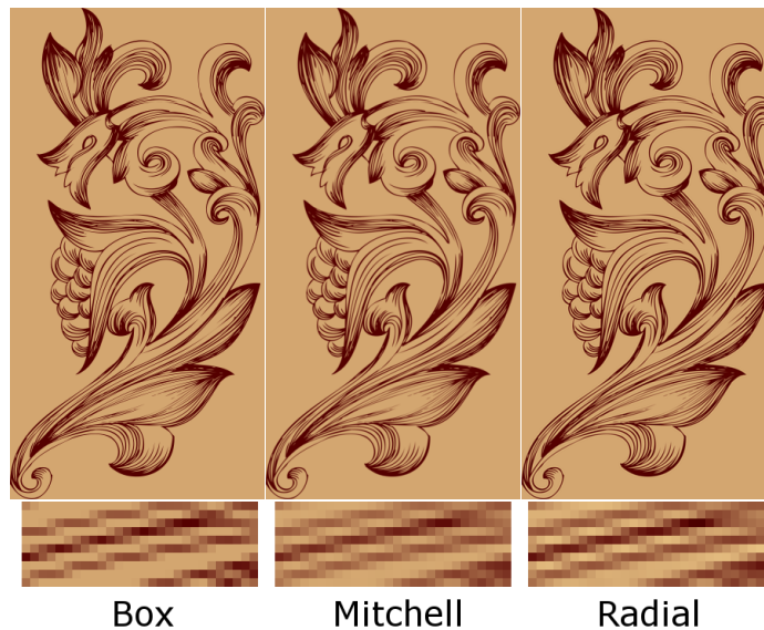
Figure 2.13: An image rasterized using a box filter (left), a Mitchell-Netravali filter (center), and a radial filter of radius 3 (right). A zoomed-in section of the image is shown below each high-resolution image to show differences in pixel values.
