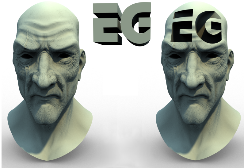
Figure 3.4: Image obtained when we used our method to calculate the CSG set difference between the head and the Eurographics logo using an anti-aliased rasterization of each model on a 1024^3 grid.
