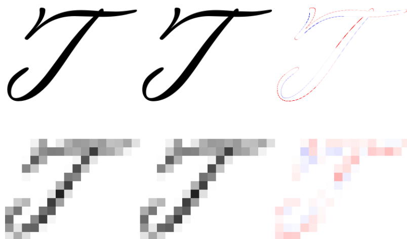
Figure 2.10: Comparison of font rendering between FreeType (left) and our Wavelet algorithm (center). In the difference image (right), red values indicate that our rendering has a higher cell coverage and blue indicates that it has a lower cell coverage. Differences are multiplied by a factor of 10 to increase visibility.
