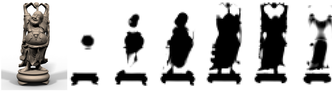
Figure 3.1: Slices from a 3D rasterization of the Happy Buddha statue computed on a 64^3 grid to illustrate the anti-aliased nature of wavelet rasterization.
