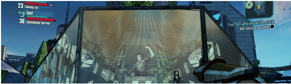
Figure 1.1: An image captured from Borderlands 2 that exhibits Moiré patterns in a billboard. Small movements create large changes to the pattern.
