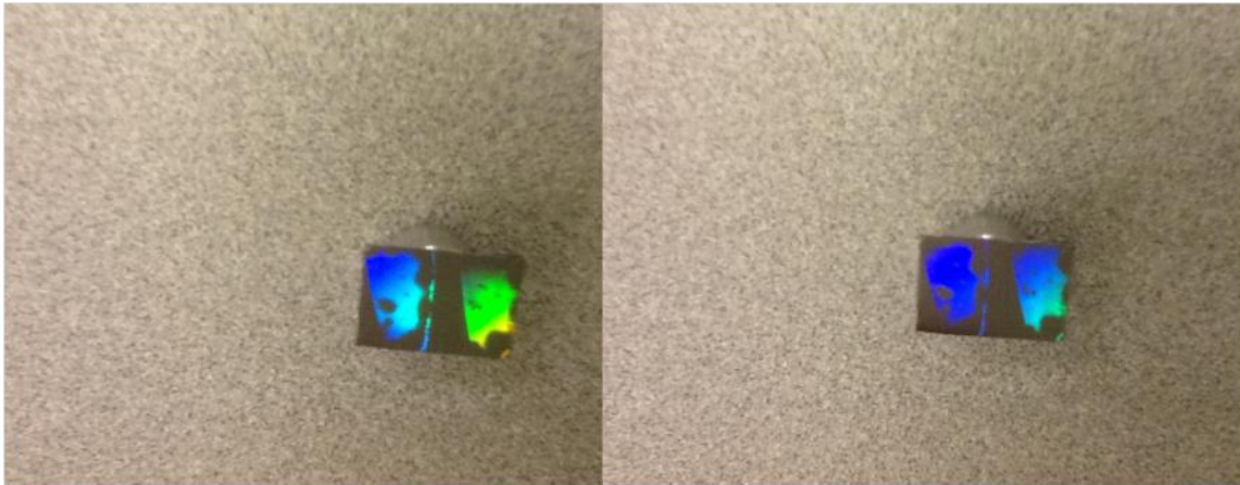
Figure 20. Photography of a substrate imprinted by two sequential steps of step-and-repeat process.
