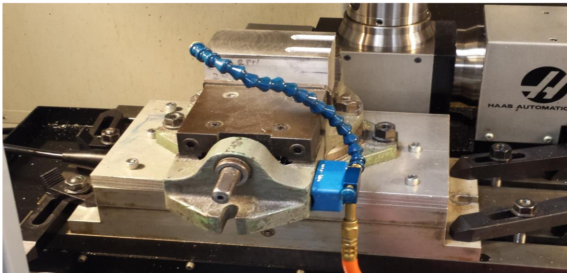
Figure 1: HAAS CNC machine with work piece mounted on a dynamometer
