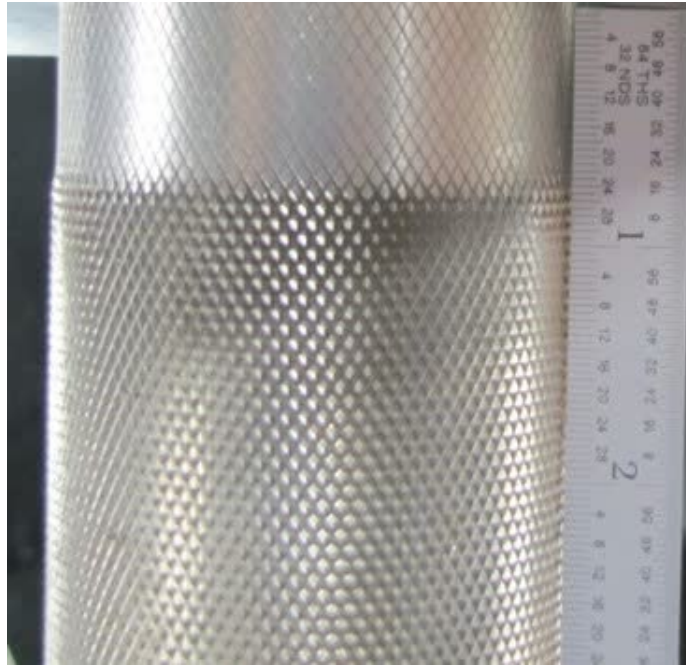
Figure A.2: Knurling on main strut
