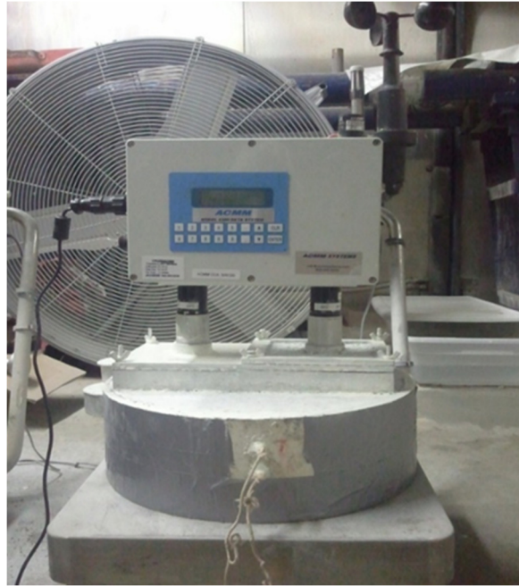
Figure 3.4: Entire Curing Monitoring System (Sun 2013)
