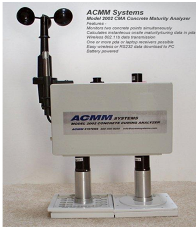
Figure 3.1: Curing Monitoring Device (Sun 2013)
