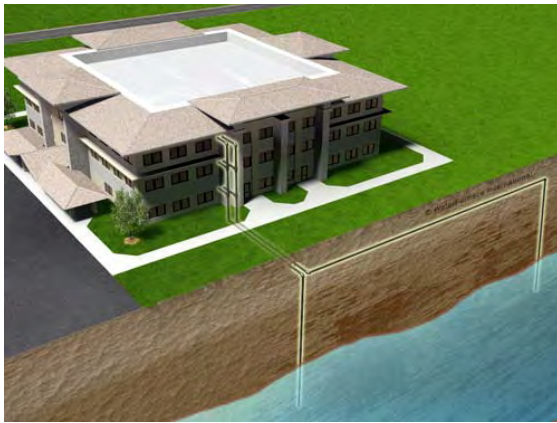
(a) Open vertical loop field
