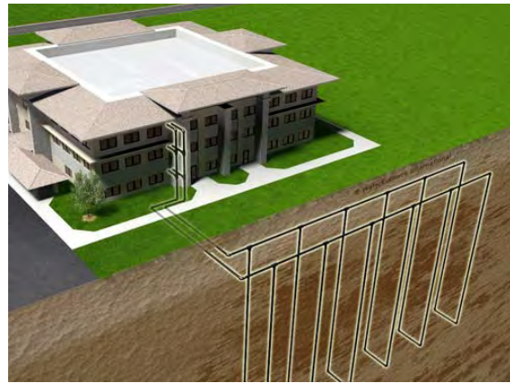
(b) Closed vertical loop field
