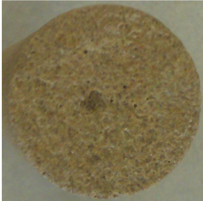
Figure IV.19: B3-3 inlet after acid injection
