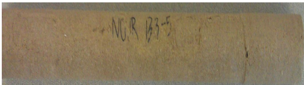
Figure IV.34: B3-5, displayed lengthwise, after acid injection
