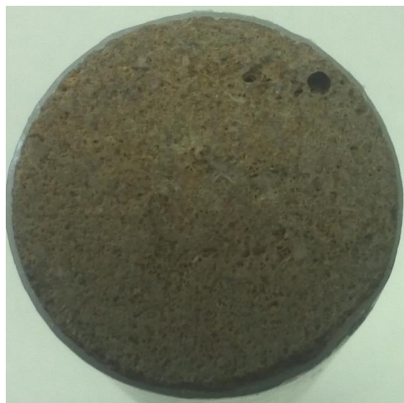
Figure III.22: B1-6 outlet after acid injection
