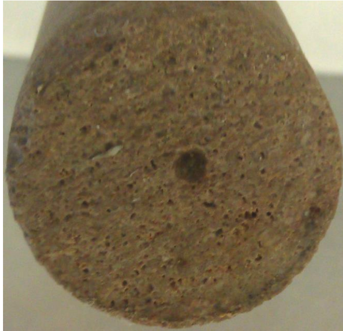
Figure IV.3: B3-1 inlet after acid injection
