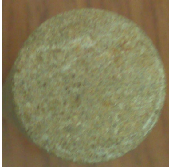
Figure IV.30: B3-5 inlet before acid injection
