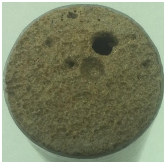
Figure III.21: B1-6 inlet after acid injection
