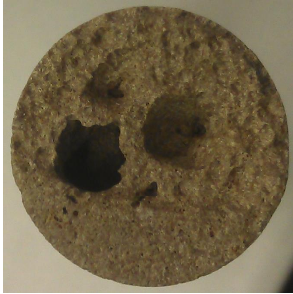
Figure IV.26: B3-4 inlet after acid injection
