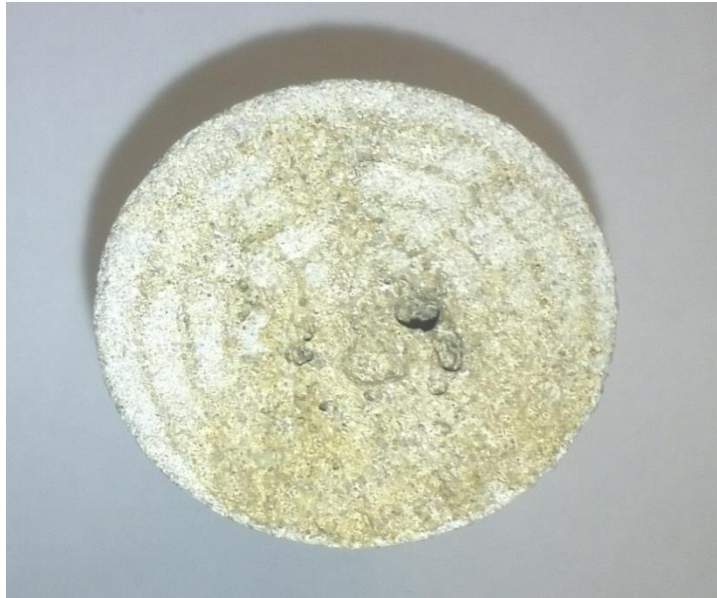
Figure III.1: B1-1 inlet after acid injection
