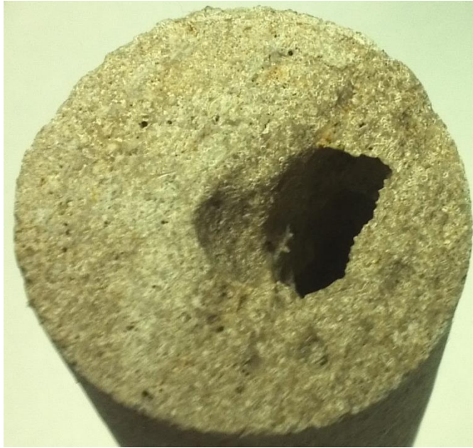
Figure III.30: B1-9 inlet after acid injection
