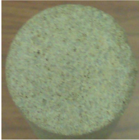
Figure IV.17: B3-3 inlet before acid injection
