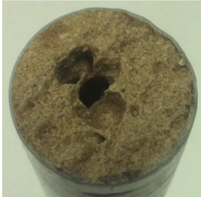
Figure III.10: B1-5 inlet after acid injection
