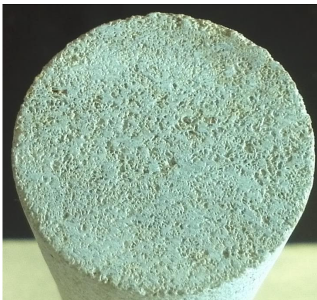
Figure III.19: B1-6 inlet before acid injection
