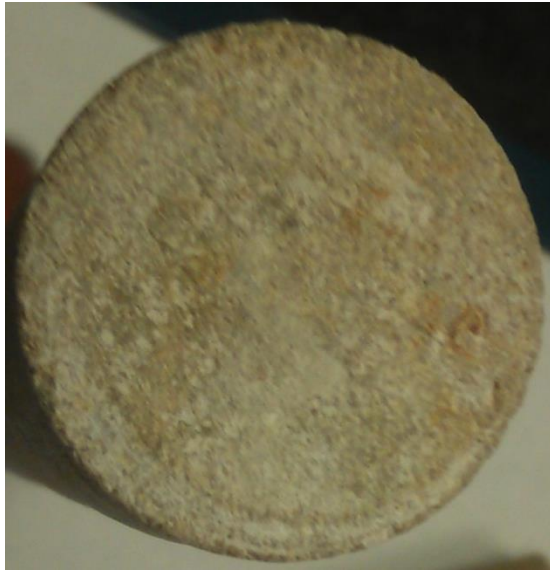
Figure IV.24: B3-4 inlet before acid injection
