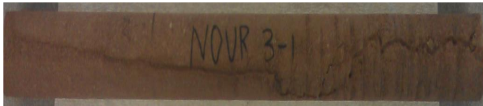
Figure IV.5: B3-1, displayed lengthwise, after acid injection
