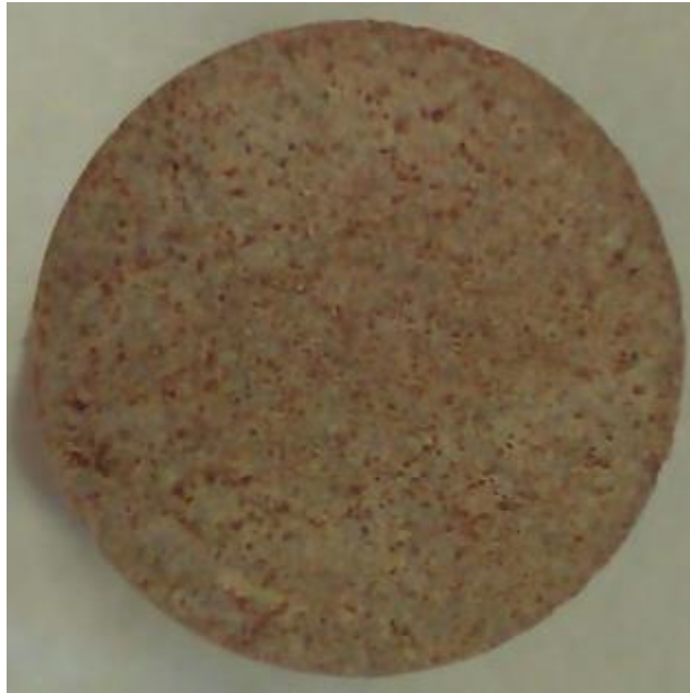
Figure IV.1: B3-1 inlet before acid injection
