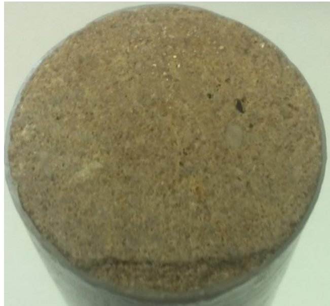
Figure III.11: B1-5 outlet after acid injection
