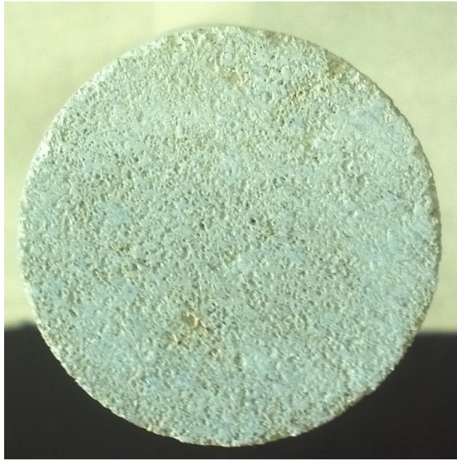
Figure III.8: B1-5 inlet before acid injection
