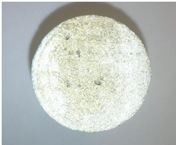
Figure III.2: B1-1 outlet after acid injection
