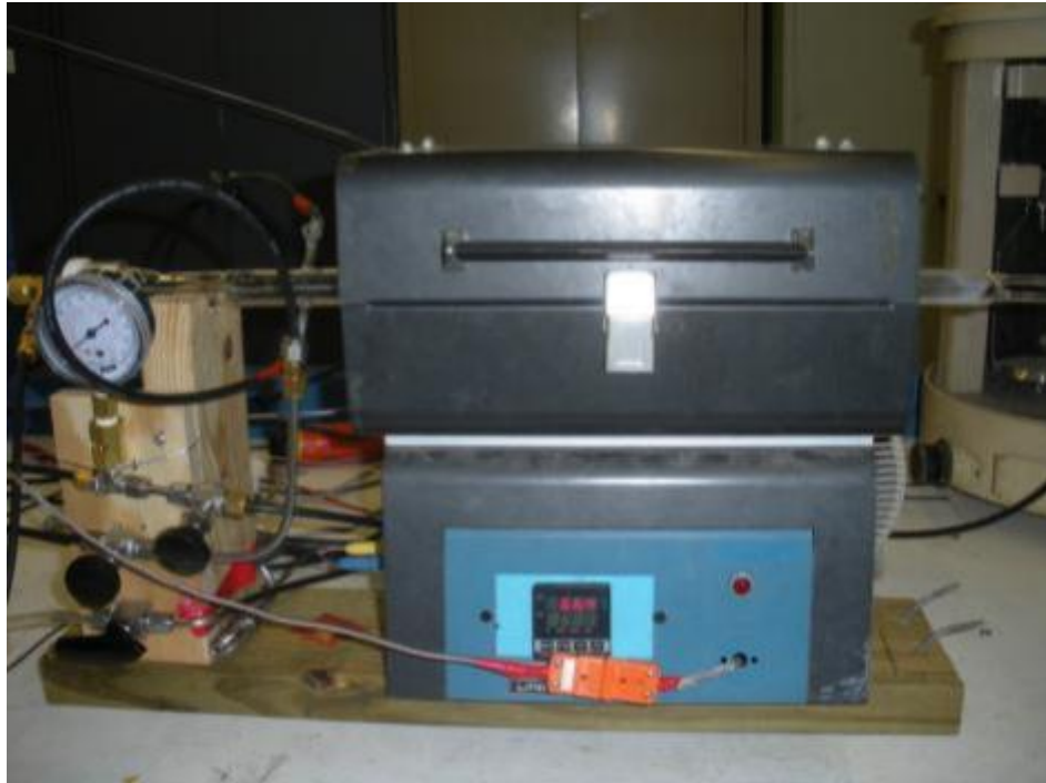
Fig. 42: Lindberg furnace with quartz tube for heat treatment processing.
