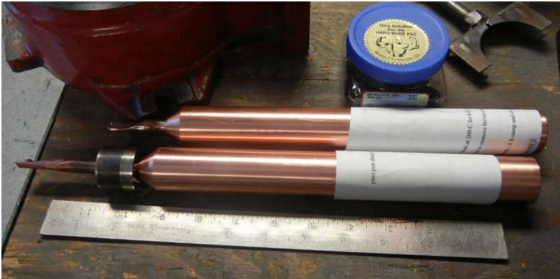
Fig. 28: Fully assembled, sealed billets with carbide die over evacuation tube.
