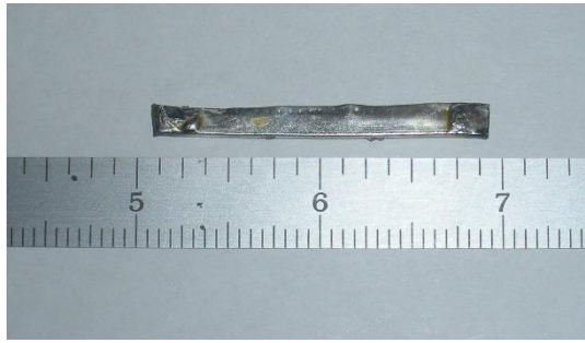
Fig. 37: Encased sample from early transport measurement attempts with sintered 1 mm x 1 mm bar encased in a coined Ag foil.
