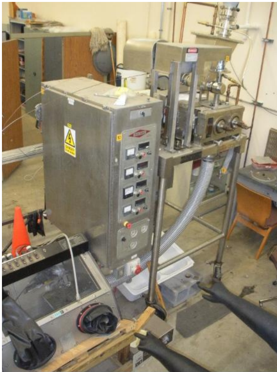
Fig. 18: Installed L-83 Chilsonator (left) and mechanical schematic of the roll processing unit (right). The glovebox in the image (left) enables a positive or negative pressure to be maintained for during operation, maintaining the hermetic seal on the output. © 2011 IEEE
