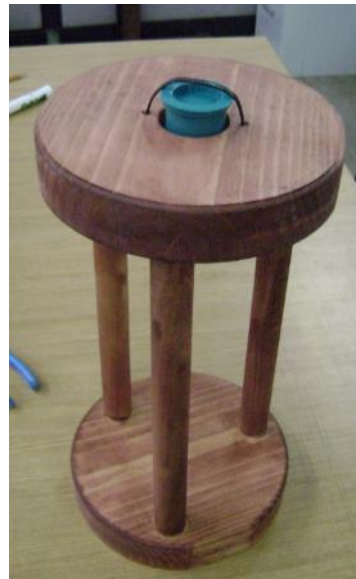
Fig. 6: Epoxy sample cup with mixed Bi-2212 powder on non-magnetic sample holder. The magnetic field would be oriented vertically (parallel to the supporting dowels) in this image.
