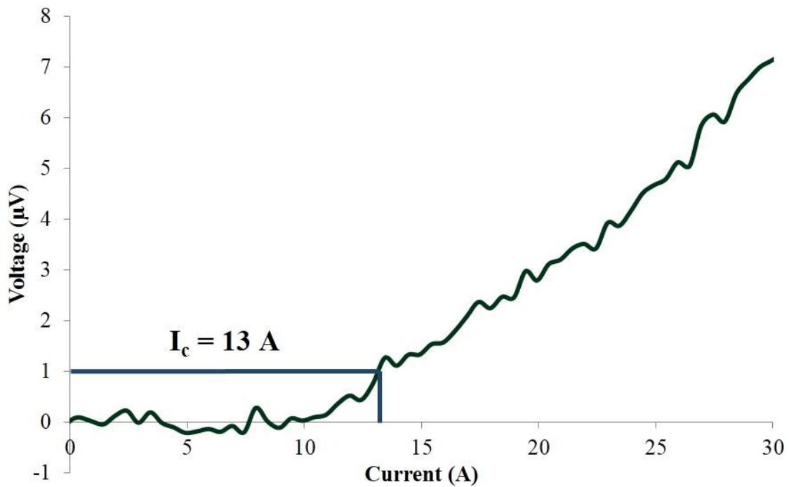
Fig. 54: V vs. I curve of highest performing TPC.
