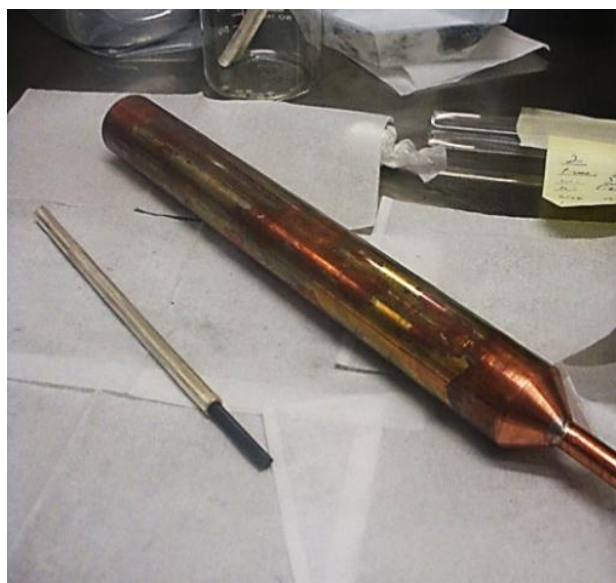
Fig. 26: Billet components during assembly including Cu extrusion jacket, Ag tube, and coined Bi-2212 rod partially inserted into the Ag tube.
