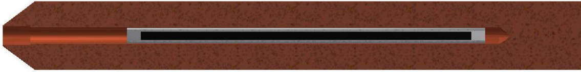
Fig. 27: Cross sectional view of assembled billet showing from interior to exterior the placement of the Bi-2212 rod, Ag tube, and Cu extrusion jacket. The evacuation tube and Cu plugs are omitted for clarity.
