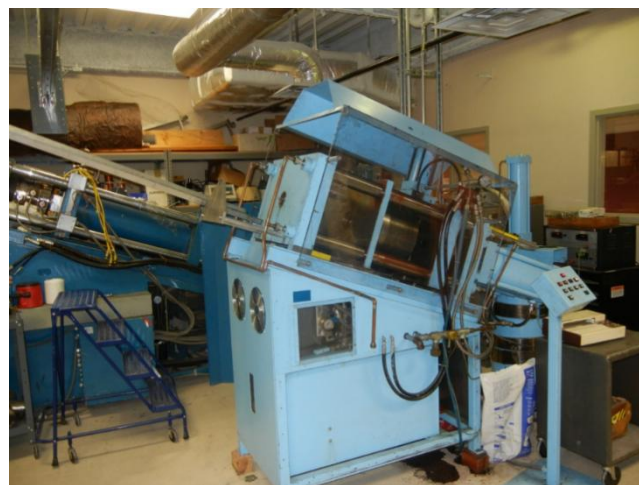
Fig. 30: Isostatic extrusion press at ASC. Billets are loaded through the opening at left into the extrusion chamber. The chamber is flooded with hydraulic fluid, and pressurized until the billet seals on the die. Continued increase in hydraulic pressure extrudes the billet.
