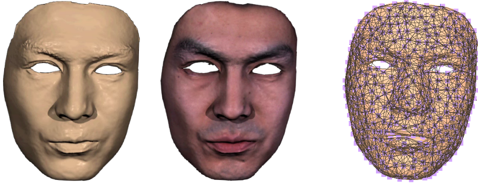
Figure 2.4: Initial template model obtained from a Minolta VIVID 910 laser scanner under a neutral expression. (left) scan mesh; (middle) textured scan mesh; (right) embedded deformation representation using 374 graph nodes represented by cubes.
