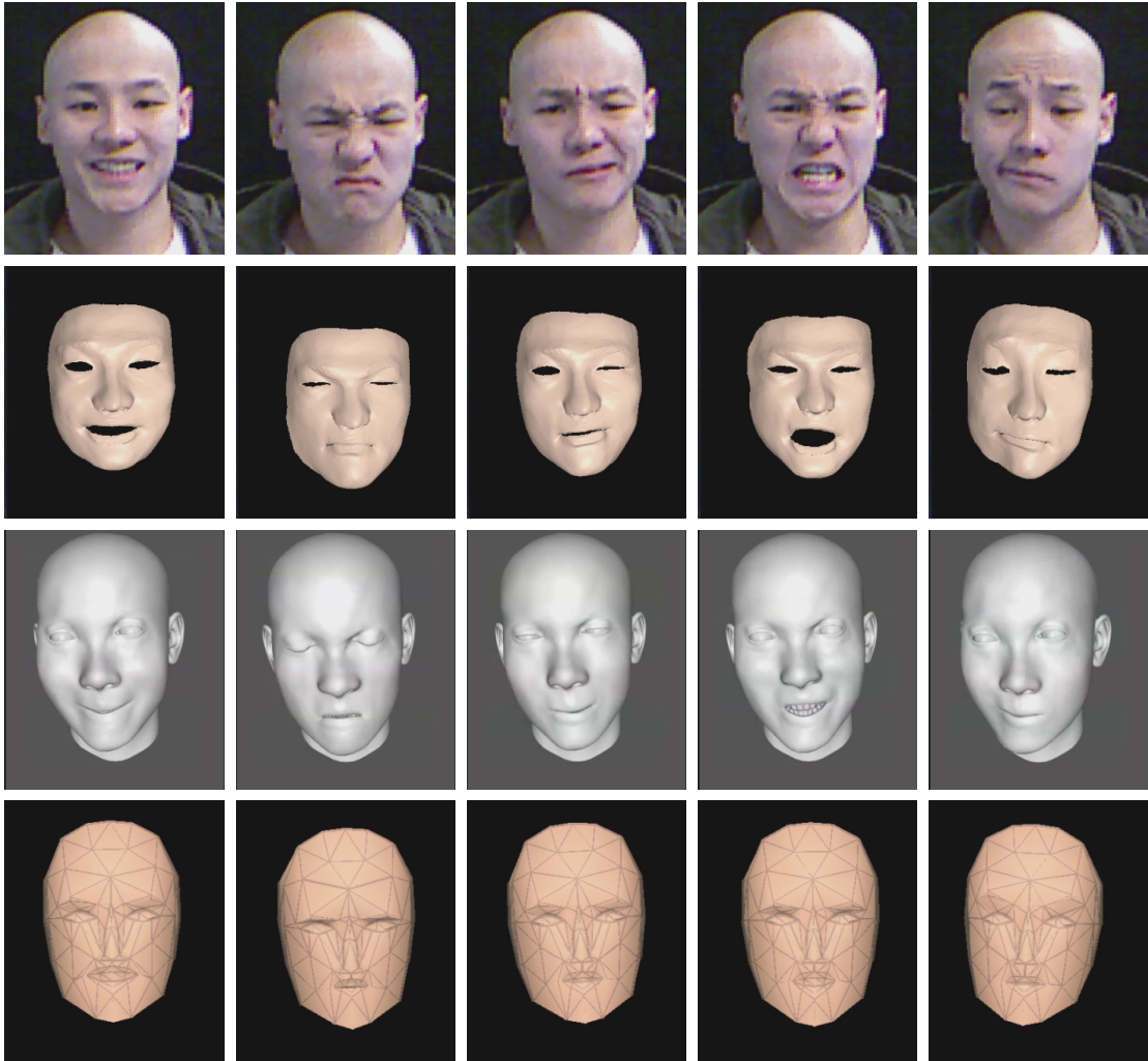
Figure 2.17: Comparisons against Weise et al. [36] and Microsoft Kinect Facial SDK [25]. Row (1) shows the reference images, row (2) shows our results, row (3) shows the results from Weise et al. [36], and row (4) shows the results from Microsoft Kinect Facial SDK [25].
