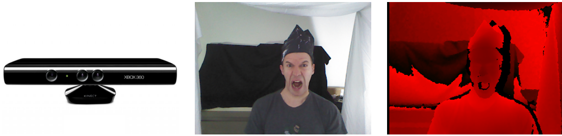
Figure 1.1: The Kinect camera simultaneously captures a 320 \times 240 pixels depth map and a 640 \times 480 pixels color image at 30 Hz.
