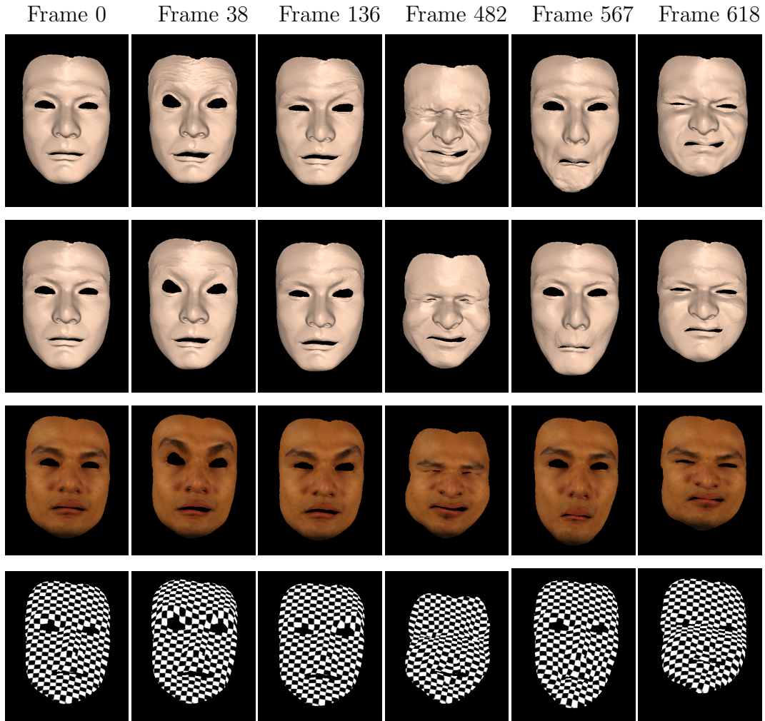
Figure 2.10: Our reconstructed results on synthetic data: row (1) shows ground truth facial performances; row (2) shows our reconstructed results; row (3) shows textured result meshes; row (4) shows result meshes with chessboard pattern.
