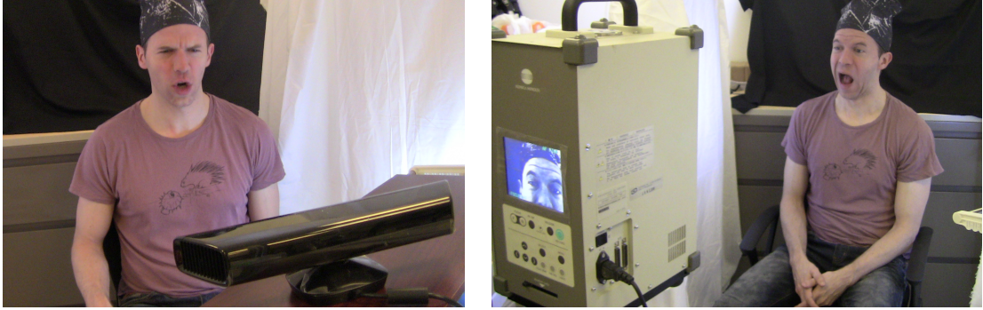
Figure 1.3: The capturing equipments and environment settings for our proposed systems. (left) a Kinect camera is used for capturing large-scale movements; (right) a Minolta VIVID 910 laser scanner is used for scanning static facial geometry of an actor to help in reconstruction of high-fidelity facial details.
