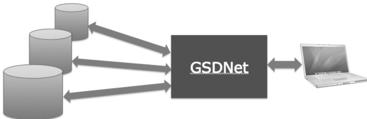
Figure 1. The GSDNet provides access to multiple data types form distributed systems, visualization tools for analysis, and data submission capability through a single user interface.
