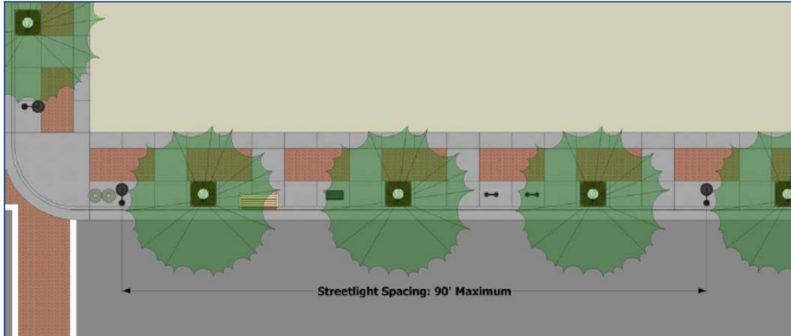
Figure 6.6 Pedestrian-scaled lamp spacing
