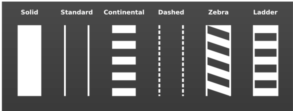
Figure 2.2 Traditional painted crosswalks
