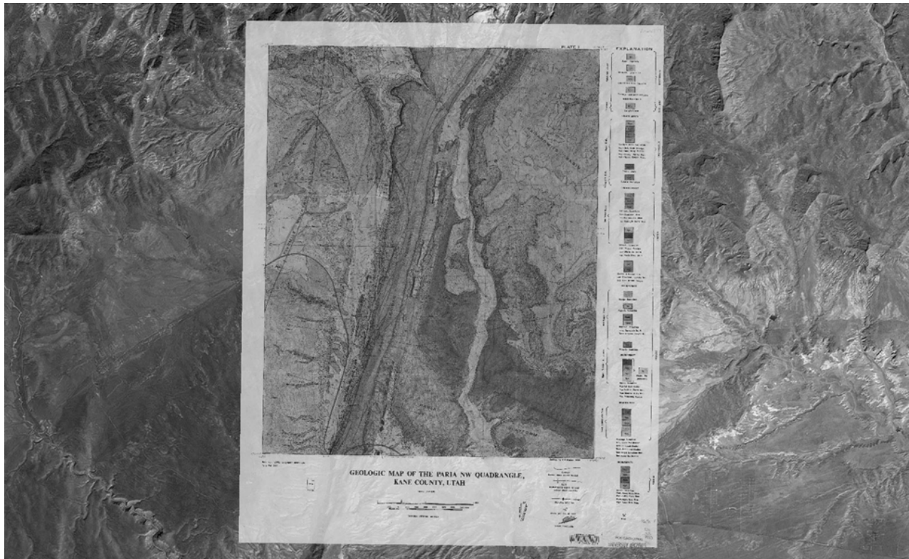
Figure 1. Example of a georeferenced map. Notice how the map overlays the topographic image and the geological features align. (Blakey, 1970)
