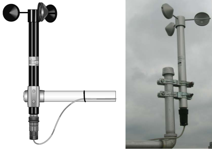
Figure 217 Anemometer Metone 014A
