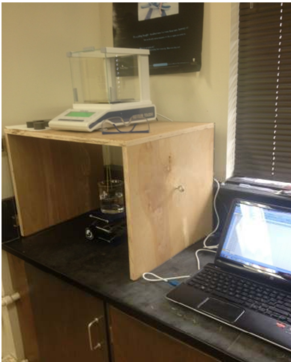
Figure 1: Experimental setup including computer for collection, balance, chamber, scissors jack, and sample in contact with a solution of interest.
