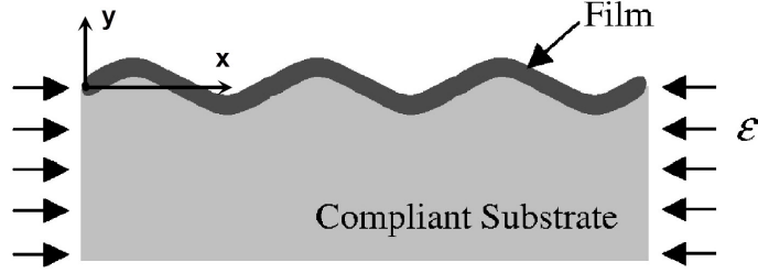
Figure 1.3: Schematic of an elastic film wrinkling on a compliant substrate (Huang et al., 2007)
