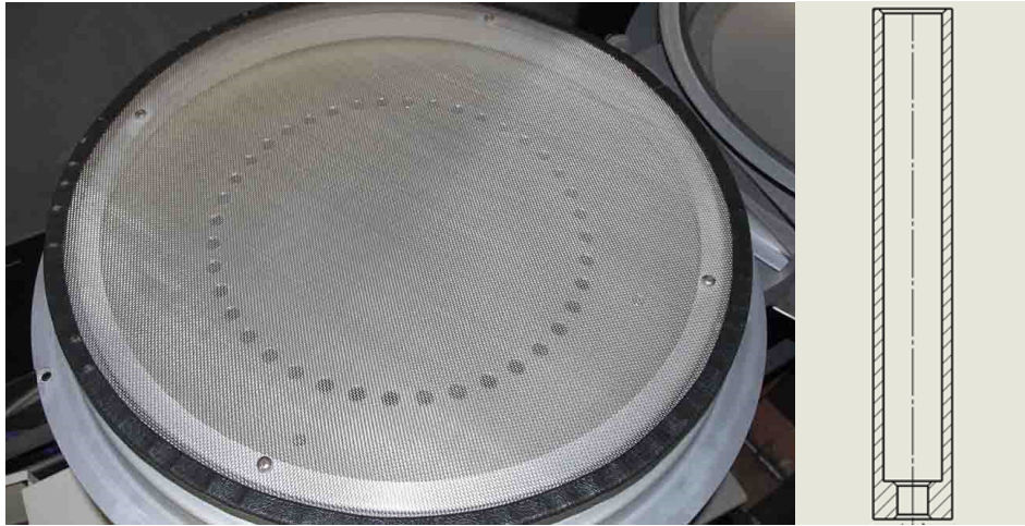
Figure 2. Retrofit nozzle bank with 40 nozzles in the sampler and single nozzle profile.
