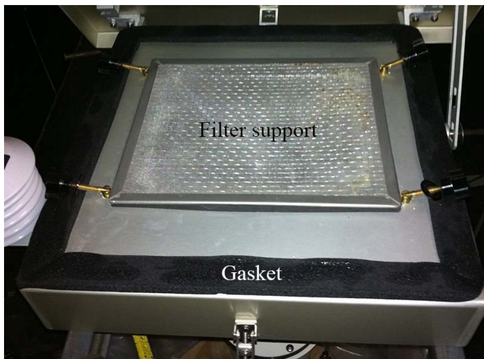
Figure 10. New gasket inside the sampler.
