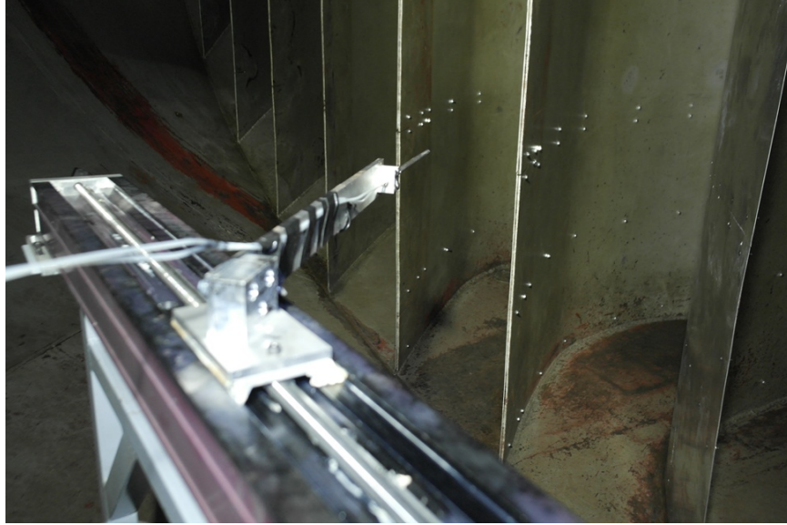
Fig. 33: Traverse mechanism behind proof of concept turning vanes.
