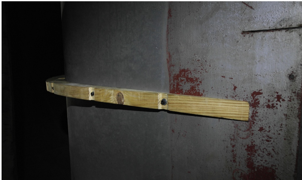
Fig. 29: Downwind section of turning vane rib modification.
