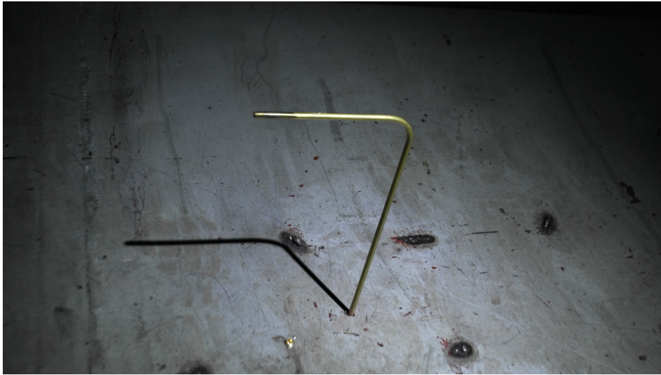
Fig. 14: Pitot tube inside tunnel, behind power section.
