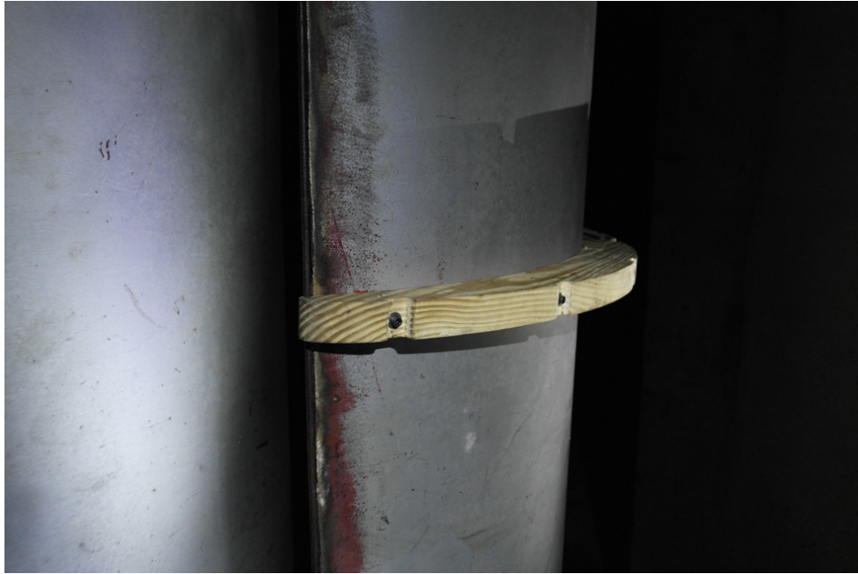
Fig. 28: Upwind section of turning vane rib modification.
