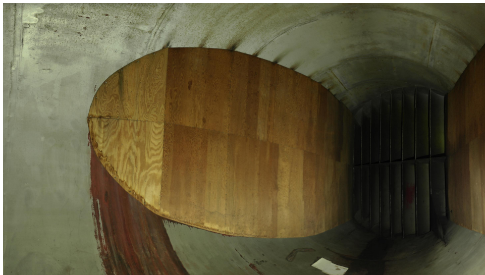
Fig. 9: View of the wood insert between turns one and two. Separation was expected here due to the relatively abrupt area change along the last 5 feet of the insert.
