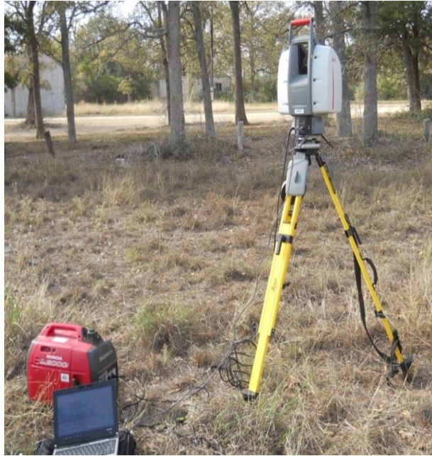
Figure 3. Leica ScanStation2, located over the center of a scanner setting at study site 1.
