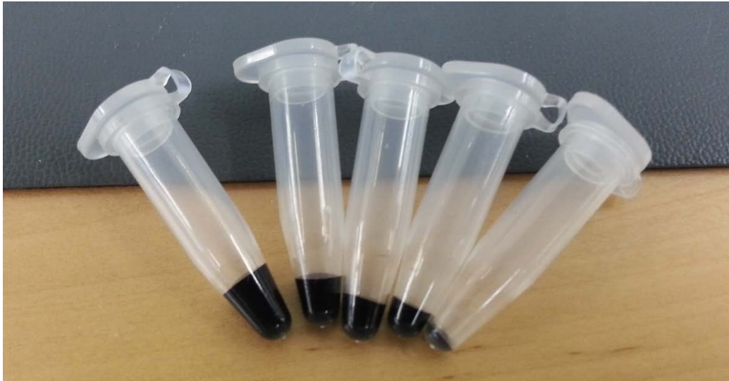
Figure IV-12 Test tubes of drops of SPIO, going from left to right we have 7, 4, 3, 2 and 1 drop.
