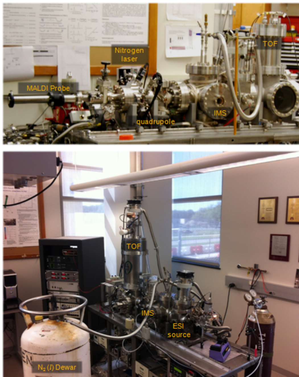
Figure 33. Photographs of the initial (top) and final (bottom) cryogenic IM-MS instrument apparatus.
