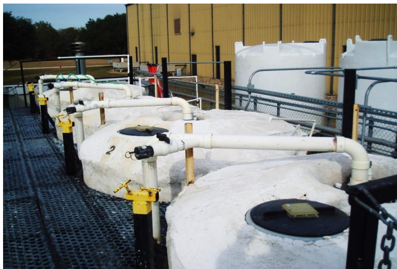
Figure 6-2. Top section of the four pilot-plant fermentors including the cat-walk.
