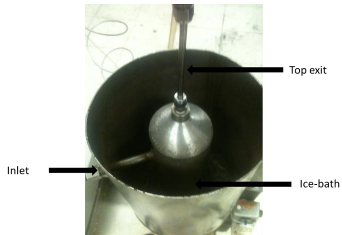
Figure 2-24. Photograph of the condenser.
