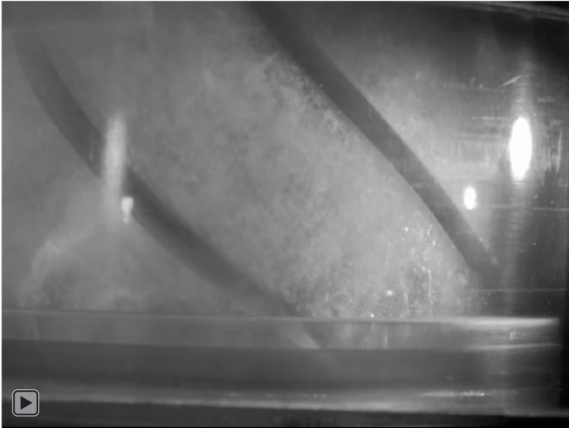
Figure 63 10,800 fps clip of diffuser inlet at 16,000 bpd flow rate and 2% GVF
