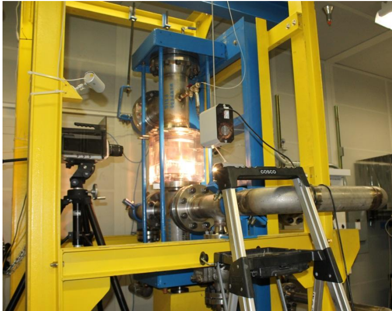
Figure 40 V711 Phantom camera and ThorLabs OSL1 light sources during testing
