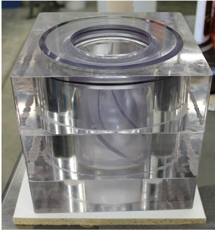
Figure 28 Pump casing with diffuser installed
