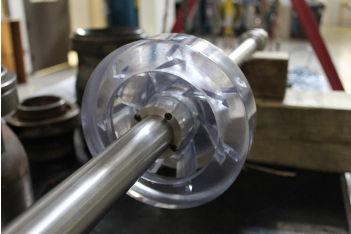
Figure 26 Impeller, collar, and shaft completed assembly
