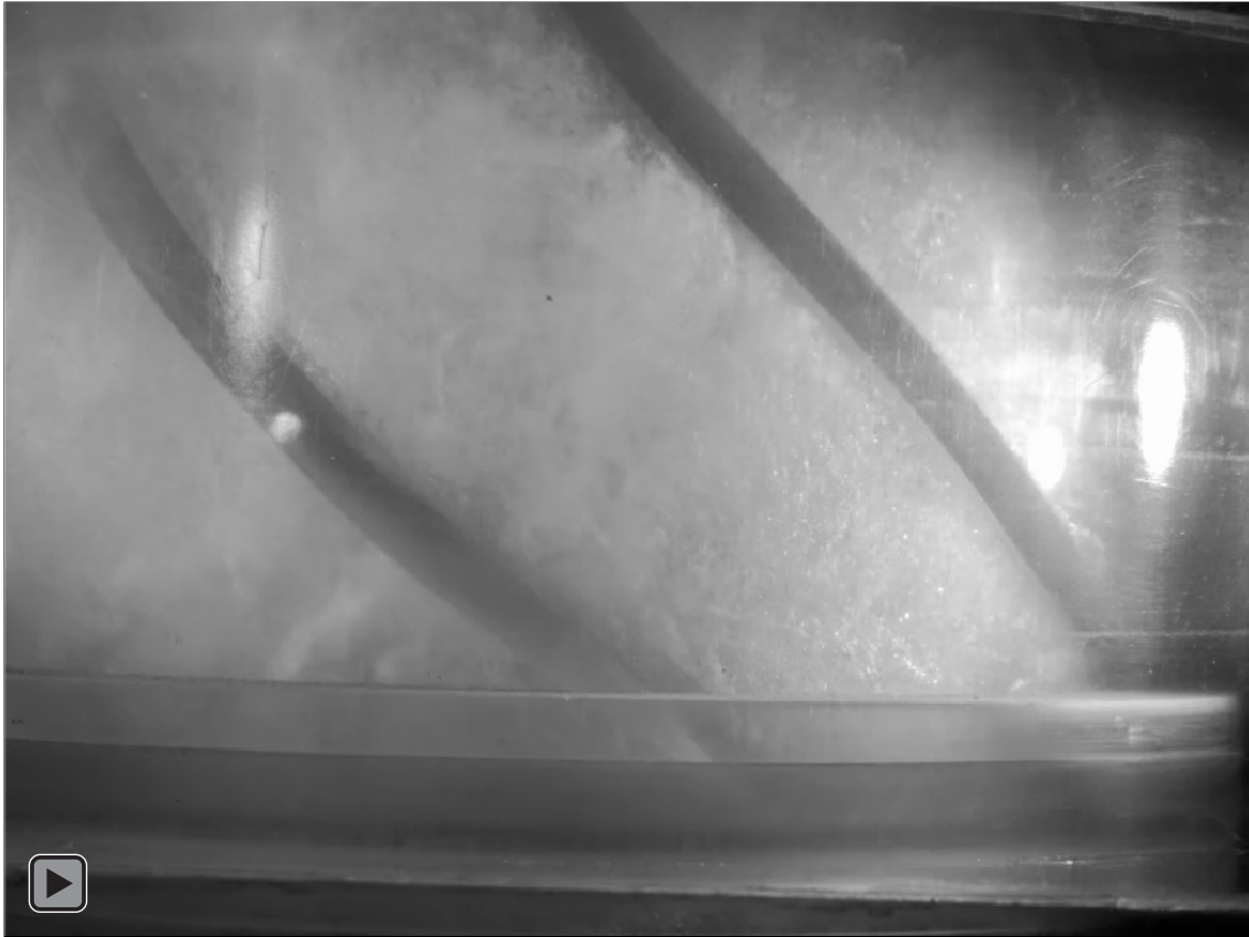
Figure 59 10,800 fps clip of diffuser inlet at 12,000 bpd flow rate and 2% GVF
