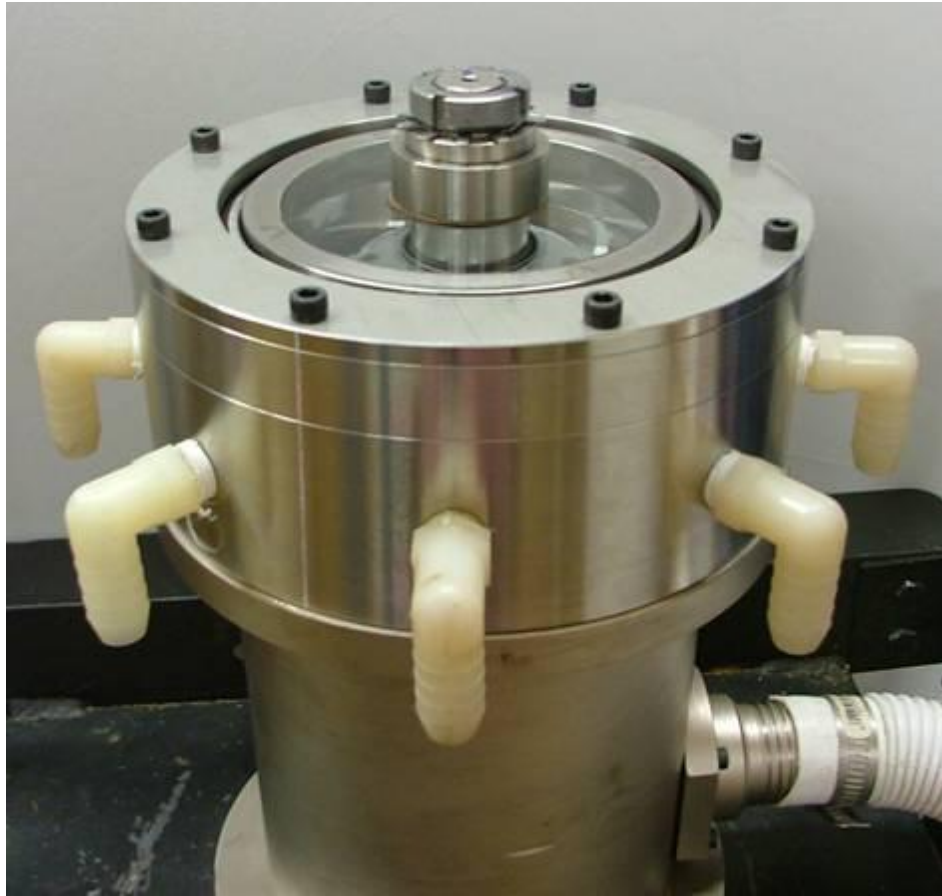
Figure 7 One-stage prototype of GC1000 conventional ESP for visualization and performance testing, Barrios [4]
