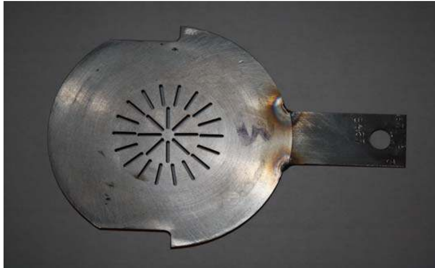
Figure 2.1 Slotted Orifice Flow Meter, \beta=0.476 .
