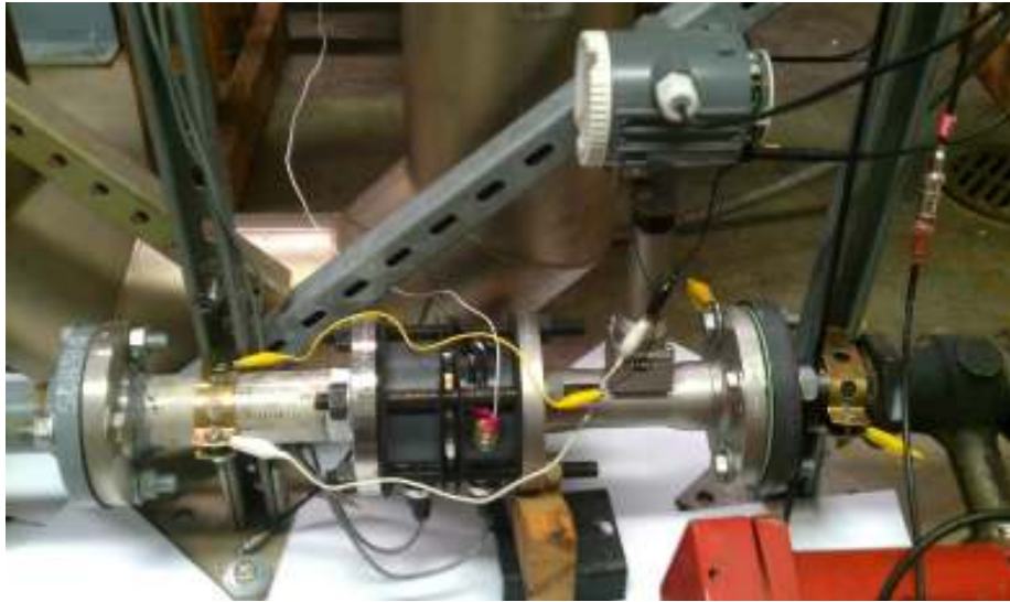
Figure 5.7 The Close Coupled Slotted Plate And Swirl-Meter.
