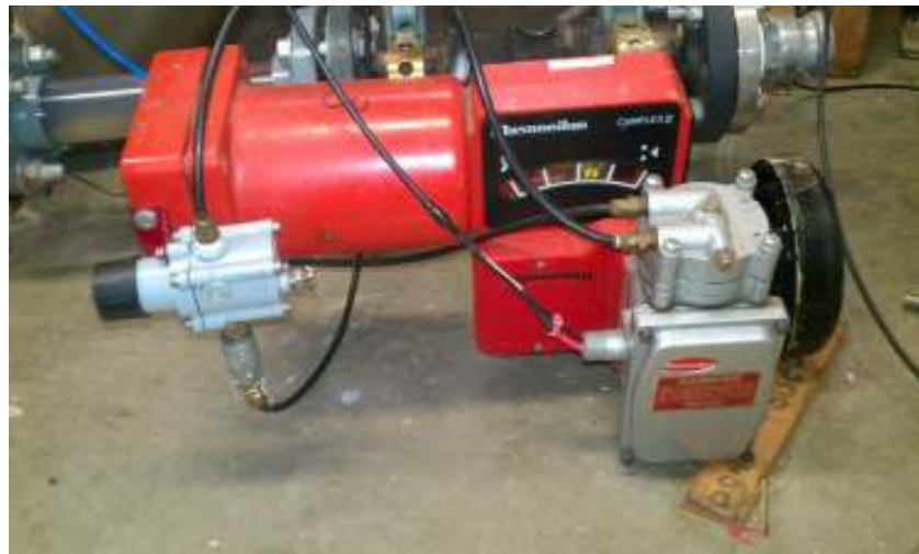
Figure 5.6 Masoneilan Control Valve.
