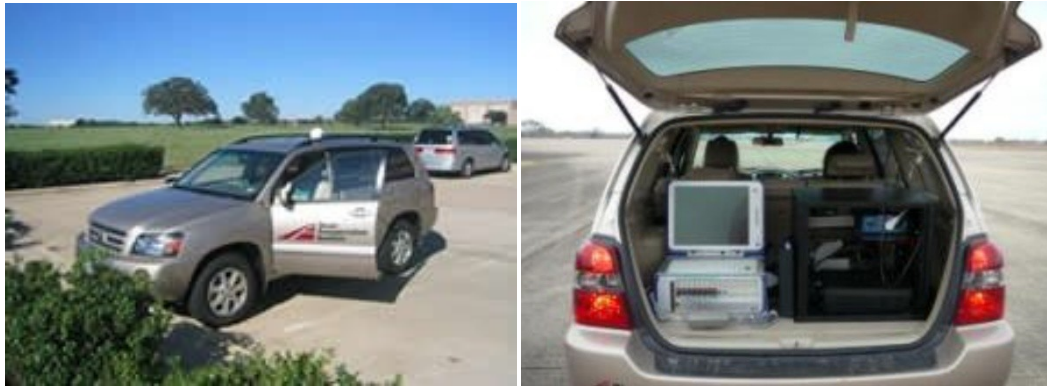
Figure 41. Instrumented vehicle and Dewetron DEWE5000 Data acquisition System
